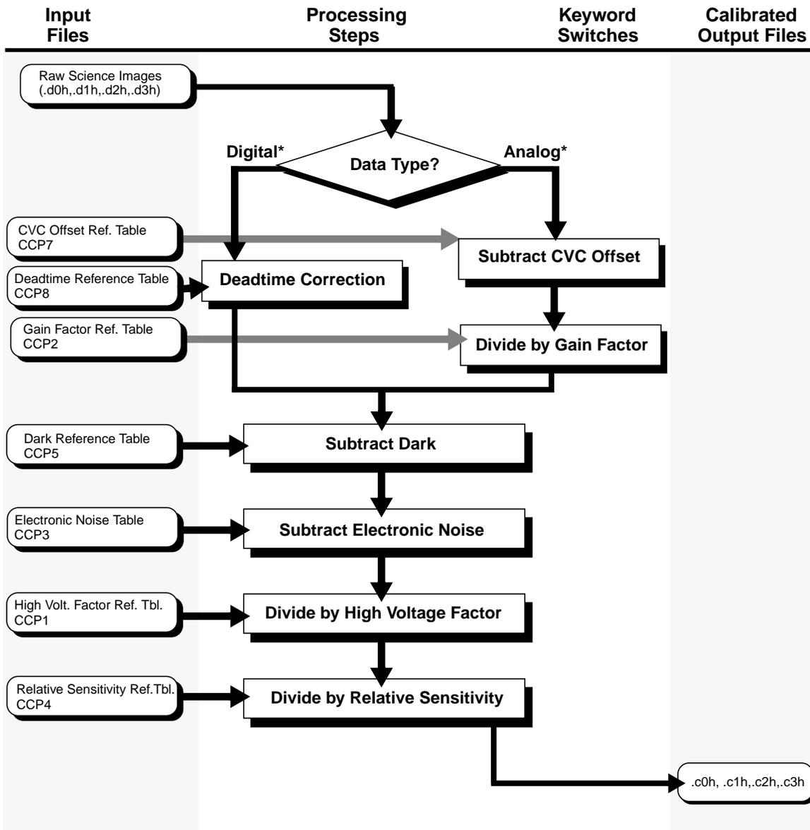
\* All **analog** steps are performed when the TRUE\_PHC switch is turned on. For **digital** data, dead time correction is turned on using the DEADTIME switch, and all other steps are turned on using the TRUE\_PHC switch.
