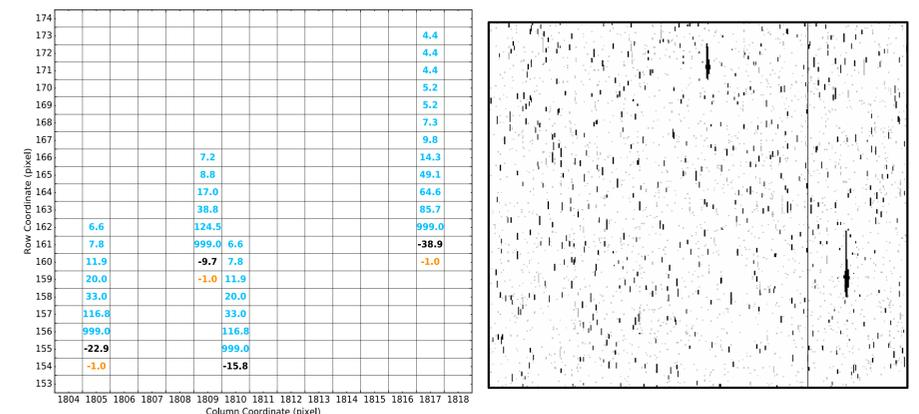
**Figure 4:** (left) A section of the Sept 2016 reference image. Each square is a pixel. Black numbers are sink pixel depths, orange numbers are high downstream pixels, and blue numbers are upstream trails. (right) A section of a science image DQ extension showing flagged sink pixels and trails (vertical dashes) and other flags.
