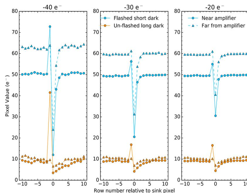
**Figure 3:** Column profiles of sink pixels with depths of  $-40 \pm 5$ ,  $-30 \pm 5$ , and  $-20 \pm 5 e^-$  (left to right). Triangles (Circles) are sink pixels in the half of the detector near to (far from) the amplifier. Blue curves are from the short dark and orange curves are from the un-flashed long (1000s) dark from the Oct. 2015 anneal cycle.
