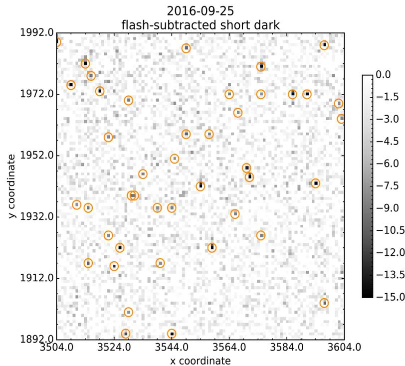
**Figure 1:** A 100x100 pixel region in the flash-subtracted short dark for the Sept. 2016 anneal cycle centered on a deep SP with a trail extending towards the top of the image.
