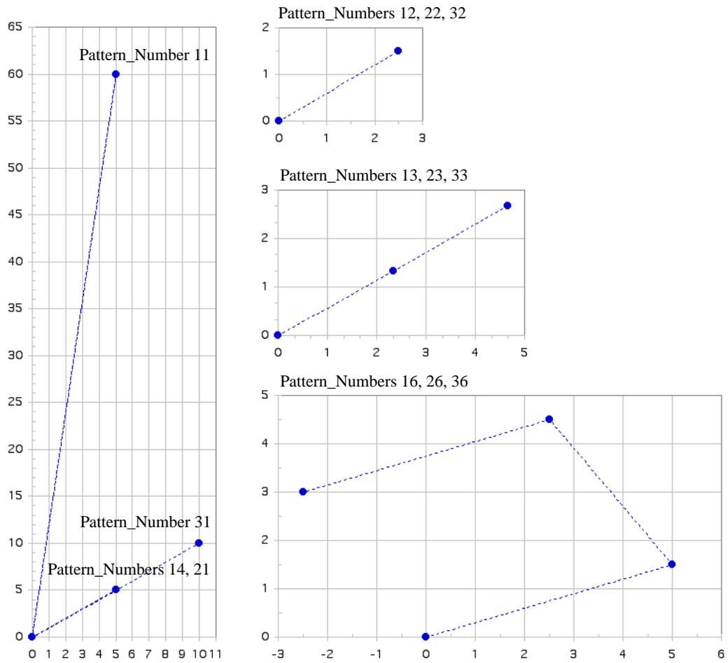
**Figure 2:** Diagrams of each dither pattern in relative pixel space.
