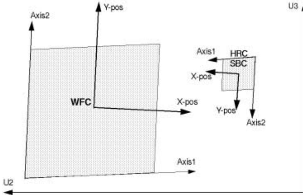
**Figure 1:** The relative orientations of the detector pixel axes (AXIS1, AXIS2), telescope pointing axes (X-POS, Y-POS), and the HST focal plane axes (U2, U3). This graphic does not reflect the relative positions of the WFC, HRC, and SBC apertures in the HST focal plane.
