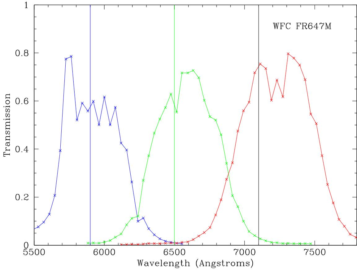
Fig. 7.— Plots of the measured transmission of the ramp filter FR647M on the WFC, set at three central wavelengths: 5900, 6500 and 7100 Å, shown by the vertical lines.
