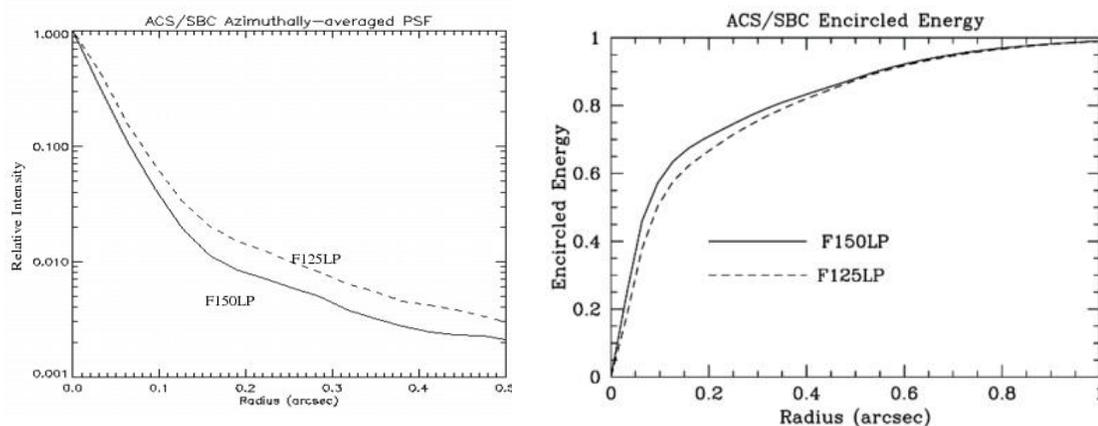
**Figure 1:** Radial profiles and encircled energy curves found in the ACS Instrument Handbook as of publication of this report. They will be replaced with the results from this work.
