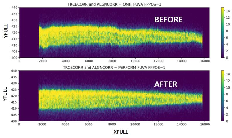
**Summary:** Illustration of the removal of the spectral trace from a FUV 2D flat-fielded image.
