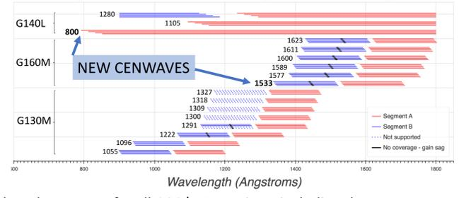
Wavelength coverage for all COS/FUV settings, including the two new cenwaves G140L/800 and G160M/1533. The four horizontal lines per cenwave indicate the FP-POS settings. The small black lines indicate gain-sagged regions.
