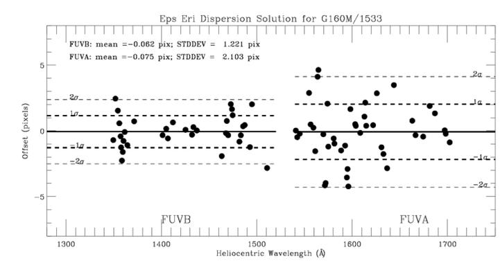
**Summary:** Illustration of the accuracy (in pixels) of the 1533 dispersion solution as a function of wavelength.
