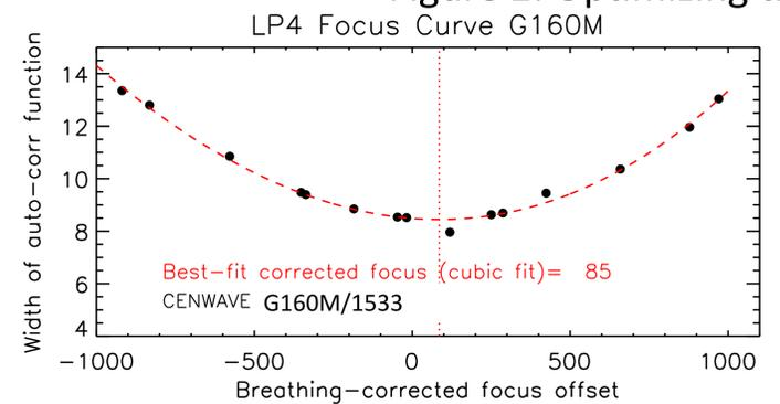
**Summary:** Focus curve for G160M/1533, showing the width of the auto-correlation function (ACF) as a function of focus position corrected for thermal breathing of the telescope.
