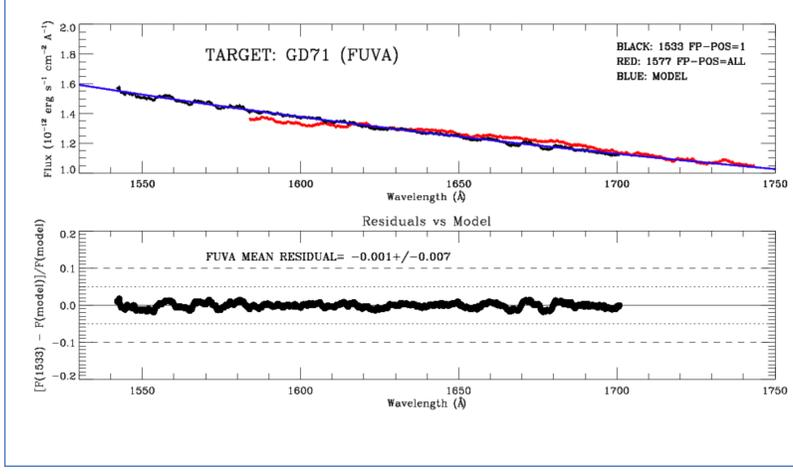
**Summary:** Illustration of the observations used to flux calibrate the 1533 cenwave on segment FUVA.
