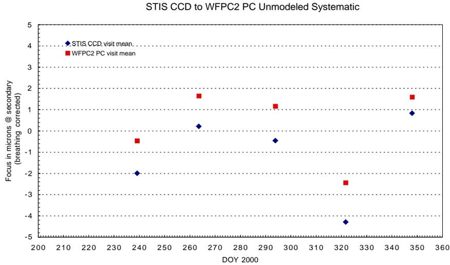
**Figure 6:** Offset between orbit means of STIS CCD and WFPC2 PC focus results.
