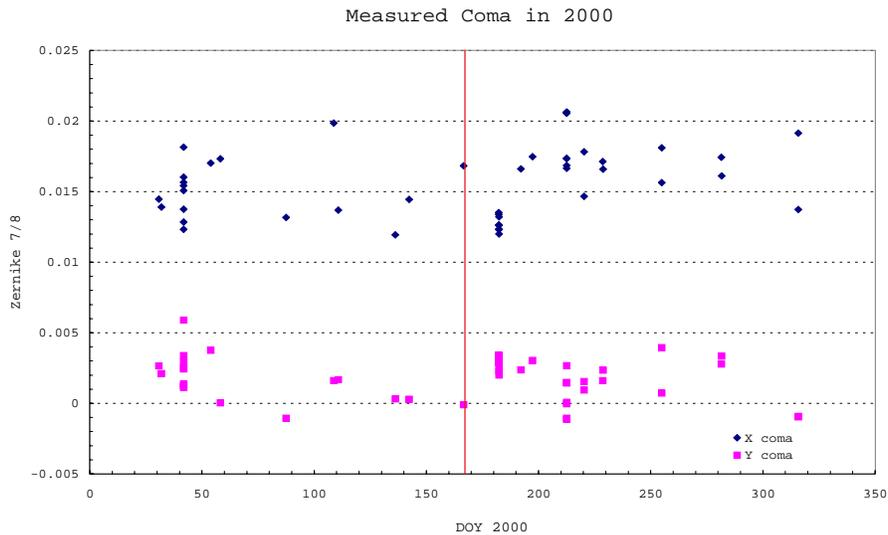
According to the stuck actuator prediction, our past three mirror moves alone should have produced a  $\Delta$  coma of 0.035, a value which is much greater than coma variations noted when comparing current numbers to data as far back as 1996.
