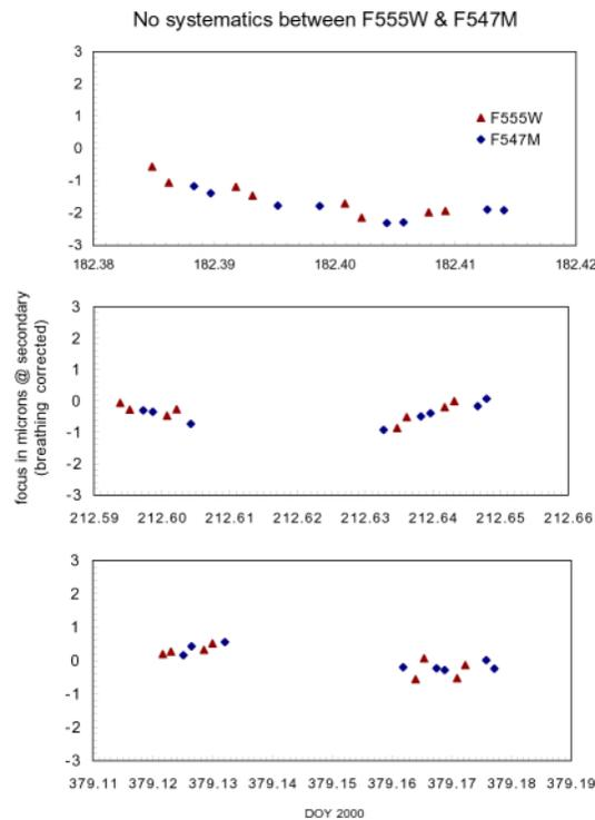
The means of the F555W and F547M sets are practically indistinguishable at  $-0.6\mu\text{m}$  and  $-0.7\mu\text{m}$  respectively, and they have comparable noise ( $0.8\mu\text{m}$  and  $0.9\mu\text{m}$   $1\sigma$  rms)
