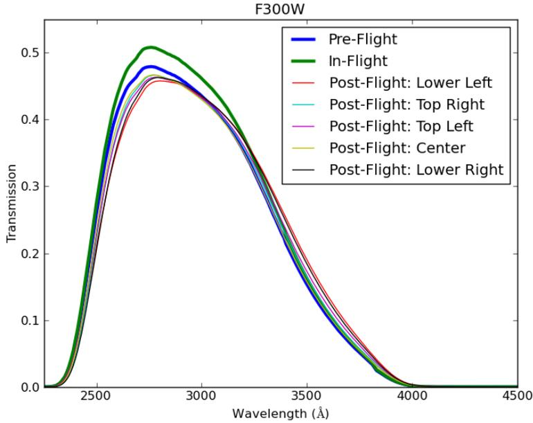
**Figure 3:** An example for FTP file category F mentioned in Section 3.1. This is a plot of F300W in-band transmission curve measurements for post-flight scan at the center of the filter. Values for peak wavelength, peak transmission, FWHM, half-max transmission, and half-max wavelengths on both sides are shown. This file is available for download from FTP<sup>7</sup> as `f300w/plots/f300w_syn_007_cen.png`.
