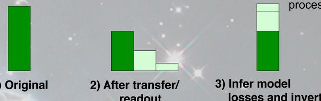
**Problem:** this can be hard to calibrate for small charge packets, where losses can be greater than 50%.
