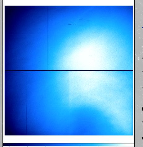
Normalized post-flash reference file for shutter A, showing the illumination pattern. Lighter indicates more illumination and darker indicates less. The post-flash pattern shows ± 20% variation across the entire FOV.
