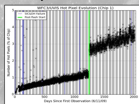
The figure to the left shows the hot pixel populations for chip 1. Time periods between anneals are represented by the gray/white regions. The green line represents the start of post-flashing the darks used to measure the hot pixel population. Prior to post-flashing,
