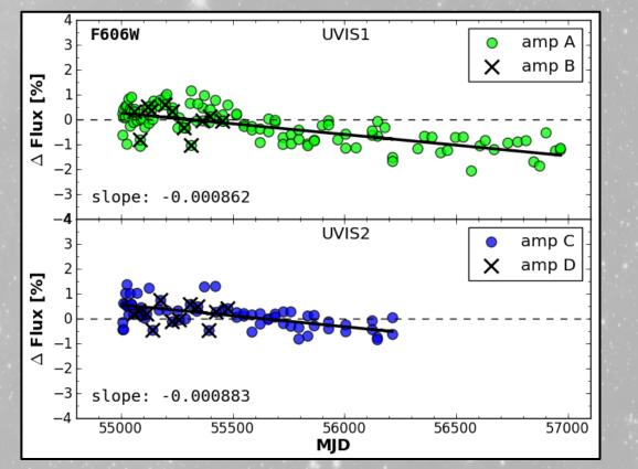
Figures: Percent difference in flux as a function of time. UV filters (e.g. F225W) show total throughput growth, while redder filters (e.g. F606W) show total throughput decline. The cause is still under investigation.
