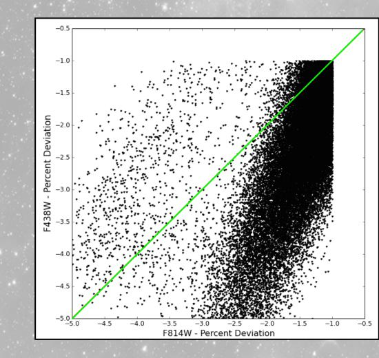
Con average the sensitivity deficit is 2 times greater in F438W than in F814W. The green line shows the 1:1 ratio of F438W and F814W. If there were no wavelength dependence, the population would be fit by this line.
