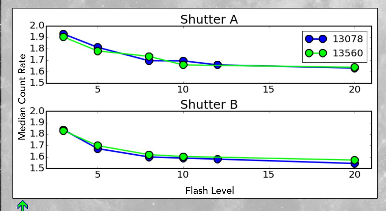
The figure above shows the median count rate as a function of flash level for both shutter blades A and B over cycle 20\* (PID 13078) and cycle 21\*\* (PID 13560). The count rate from cycle 20 through cycle 21 for both shutters is stable across all \*observation dates range 11/2012-11/2013\* \*\* observation dates range 12/2013-10/2014\*
