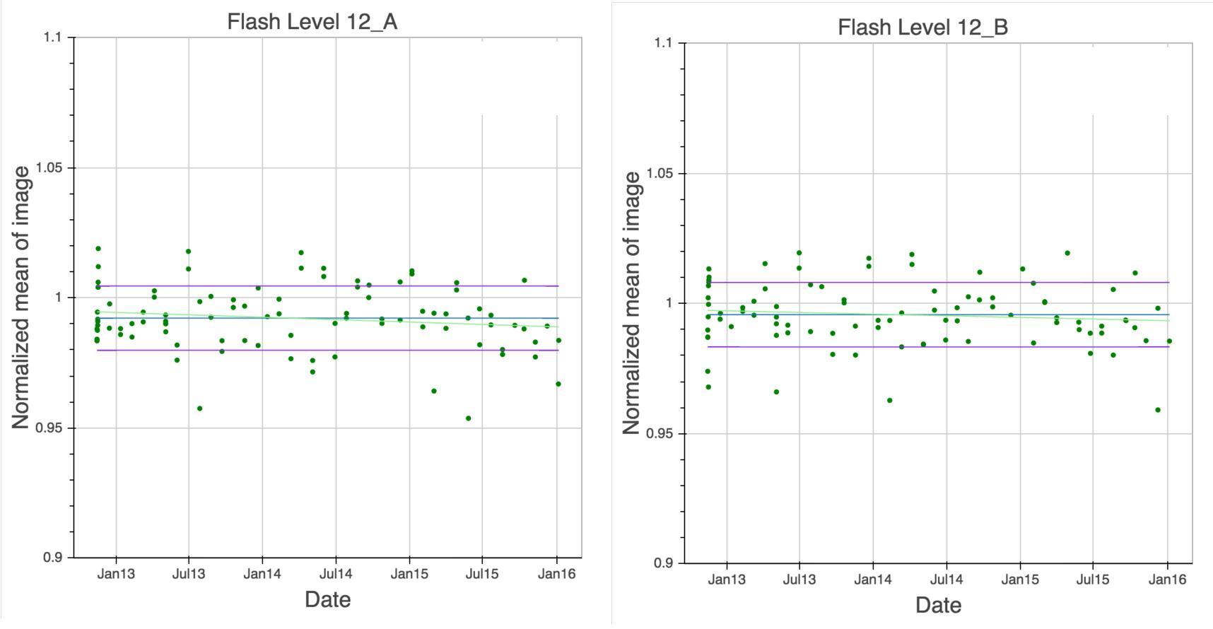
**Above:** Normalized mean post-flash over time for flash level 12 e-/pix (shutter A, B at left, right). Blue and purple lines: mean and +/- sigma, respectively. Green line is the linear fit of the data; uncertainties are less than +/- 0.05. These were made for all FLASH level/Shutter combinations.
