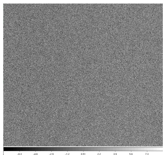
Left: Example of ratio of outlier image (ic6db3shq) to non-outlier image (ic6di3f0q). The scale goes from -8 e- to 8 e-. There are no visible patterns or shape to the ratio image indicating that there is no systematic issue causing these outliers to be dimmer or brighter than the average normalized mean measurements.
