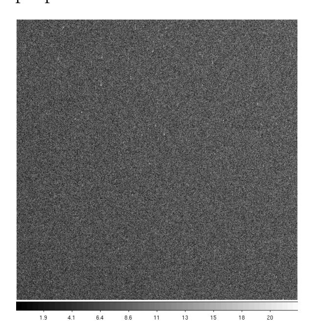
**Left:** The current normalized full frame post-flash image for shutter A. Our testing subarray is located in the lower left corner. The post-flash illumination pattern varies by  $\pm$  20% across the field.
