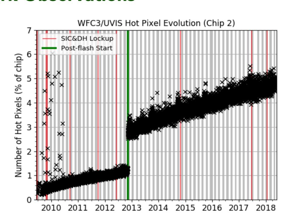
(Left) A 200x200 pixel region taken from a 900-second UVIS dark, showing the nominal features of background dark current, cosmic rays, hot pixels, and CTE trails. (Right) The number of hot pixels over time for Chip 2 (Amps C & D). ~1000 new hot pixels above the 54 e-/hr threshold appear every day, currently occupying ~5% of each chip. Each month, the UVIS detector is warmed to +20C (shaded gray/white regions) erasing 10-20% of the hot pixels.
