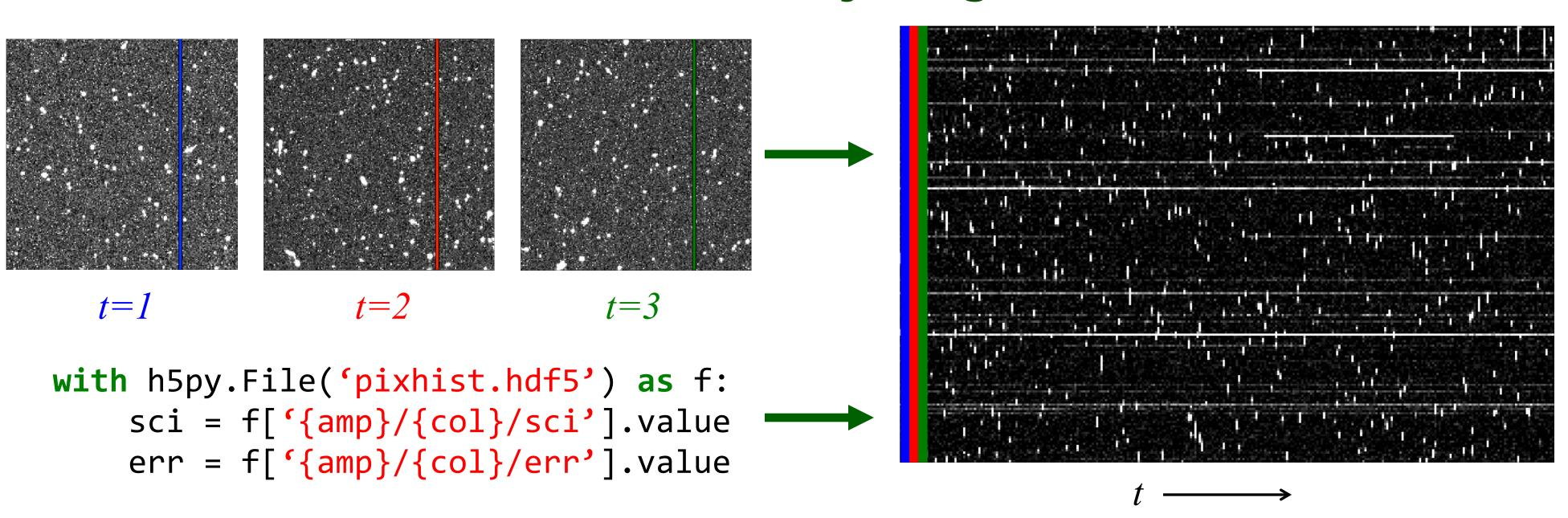
To efficiently perform pixel stability analyses, we constructed 'pixel history' images in which a single pixel's measured electron value is time-ordered along each row of the image. Each column's pixel history image was placed into a Hierarchal Data Format (HDF) dataset using Python's h5py library.
