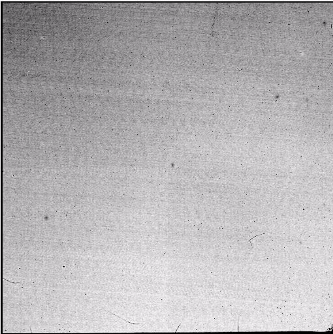
Figure 3: External F160W flatfield image from ObsID 0E. The prominent dark spots are due to dust particles on the WFC3 channel select mechanism (CSM).
