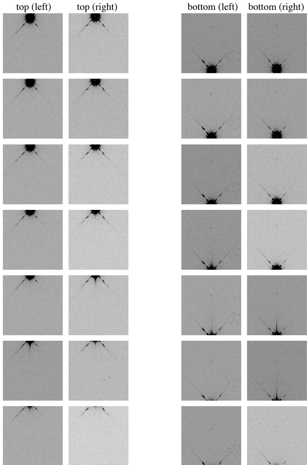
Figure 1a: A subset of positions during the baffle scans, shown as a 200x200 pixel subsection with a hard logarithmic stretch. The columns of postage stamps are for the top baffle edge (left and right sides of the detector) and bottom baffle edge (left and right side of the detector). The small glint can be seen between the diffraction spikes as the source crosses the knife edge.
