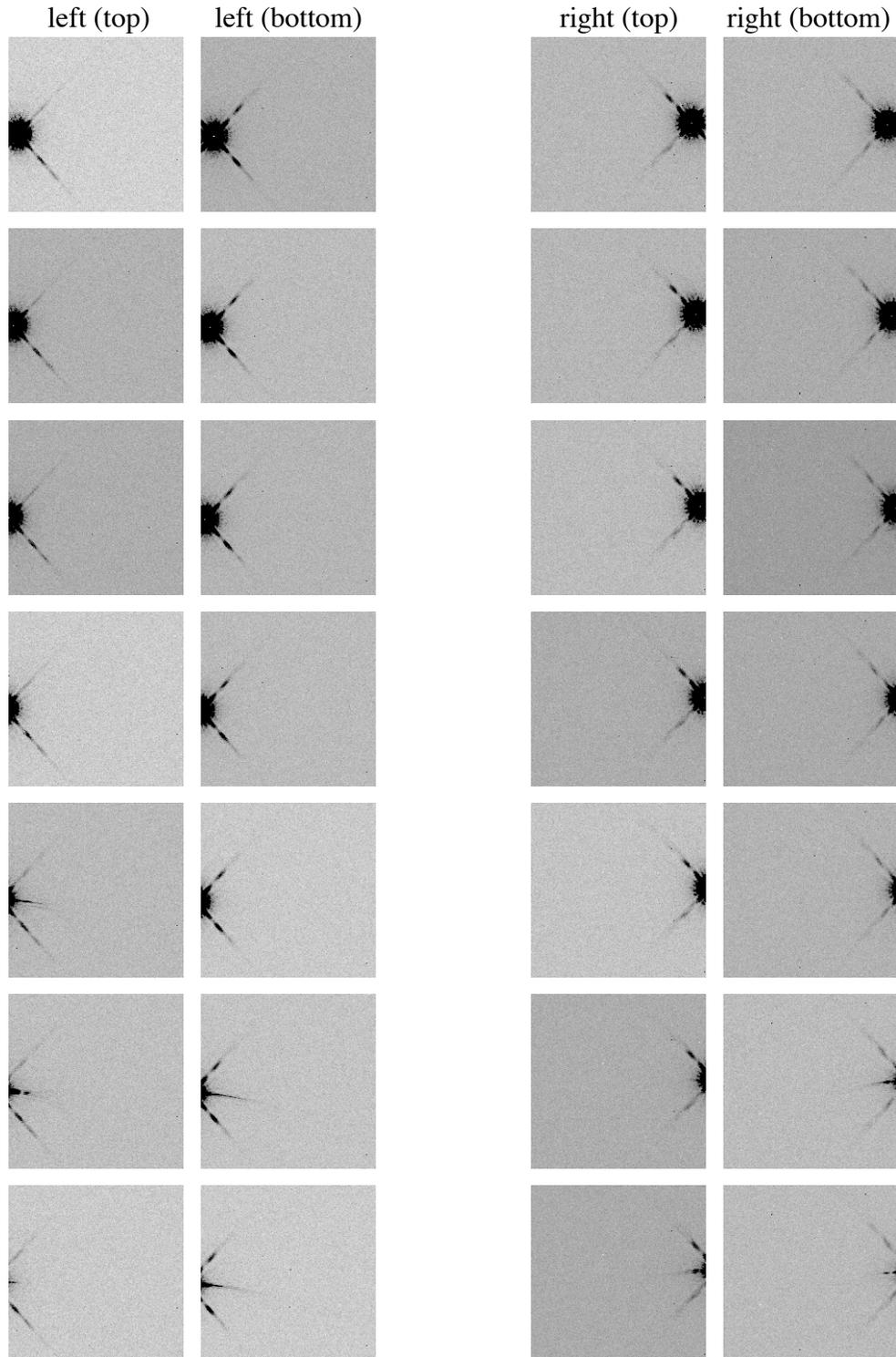
Figure 1b: A subset of positions during the baffle scans, shown as a 200x200 pixel subsection with a hard logarithmic stretch. The columns of postage stamps are for the left baffle edge (top and bottom halves of the detector) and right baffle edge (top and bottom halves of the detector). A small glint can be seen between the diffraction spikes as the source crosses the knife edge.
