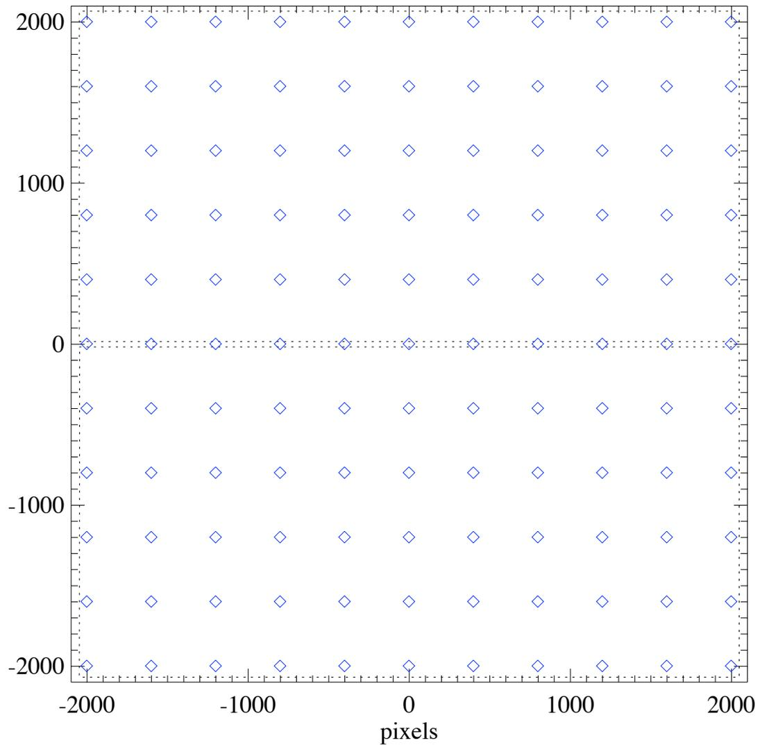
Figure 1: The positions on the UVIS detector, relative to field center, where a saturated point source was imaged for 25 seconds. The edges of the two detector halves are shown by dotted lines. A small gap (equivalent to  $\sim 34$  pixels in width) exists between the detector chips.
