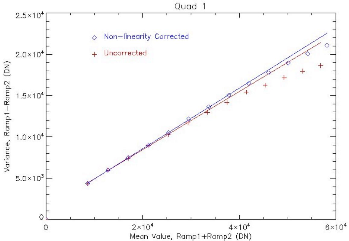
**Figure 2: Mean versus variance plot for one quadrant of one pair of ramps. The gain is the inverse of the best-fit linear slope. The red pluses show mean and variance values for a ramp without the non-linearity correction applied, while the blue diamonds show the signal values after non-linearity correction. The red and blue lines show the best-fit line to the first 5 points of the uncorrected and corrected ramps, respectively.**
