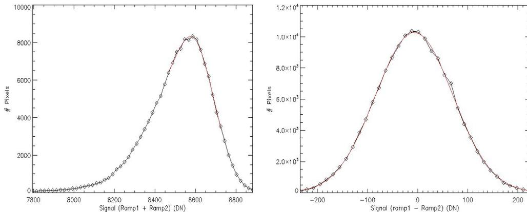
**Figure 1: Histograms and Gaussian fits of a single read of a summed (left) and differenced (right) ramp. The peak of summed histograms gave the “mean” signal values for the gain calculation, while the square of the width of the differenced histograms gave the variance values.**
