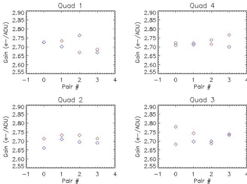
**Figure 5: Gain values calculated from data taken with MEB1. Red diamonds show values for the “first ramps” of each data dump, while blue diamonds represent the “second ramps” of each data dump.**
