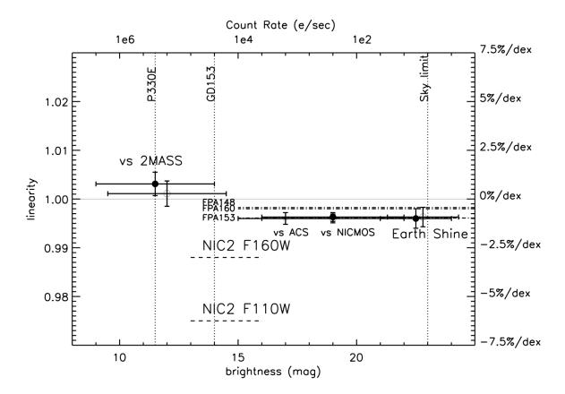
Figure 3: Comparison of assorted count-rate non-linearity measurements for WFC3-IR. The measurements reported here are labaled as "vs 2MASS" and those in Riess (2010) as "vs ACS" and "vs NICMOS". Those from Riess & Petro (2011) are labeled as "Earth Shin". Points determined from F160W are solid, from F125W are open circles and from F098M are open triangles. The values from the Goddard tested flight spares are indicated as "FPA" and those from NICMOS Camera 2 are indicated.
