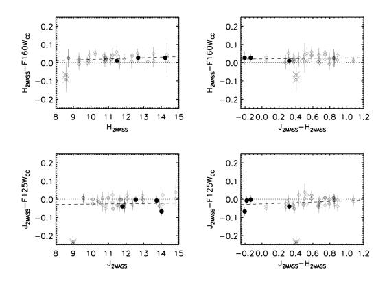
Figure 2: Photometric differences for stars between 2MASS and WFC3-IR. Asterism stars are shown as diamonds, HST standards as filled. The dotted line shows a straight line through zero residual and the dashed line shows the best fit to a 3 parameter (zeropoint difference, color residual, non-linearity) model of differences.
