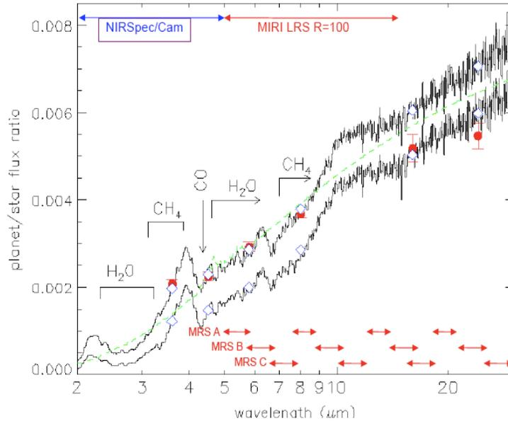
illustrated in Figure 2 from Charbonneau et al. (2008b) that shows a simulated spectrum of HD 189733b and the coverage provided by JWST's instruments.
