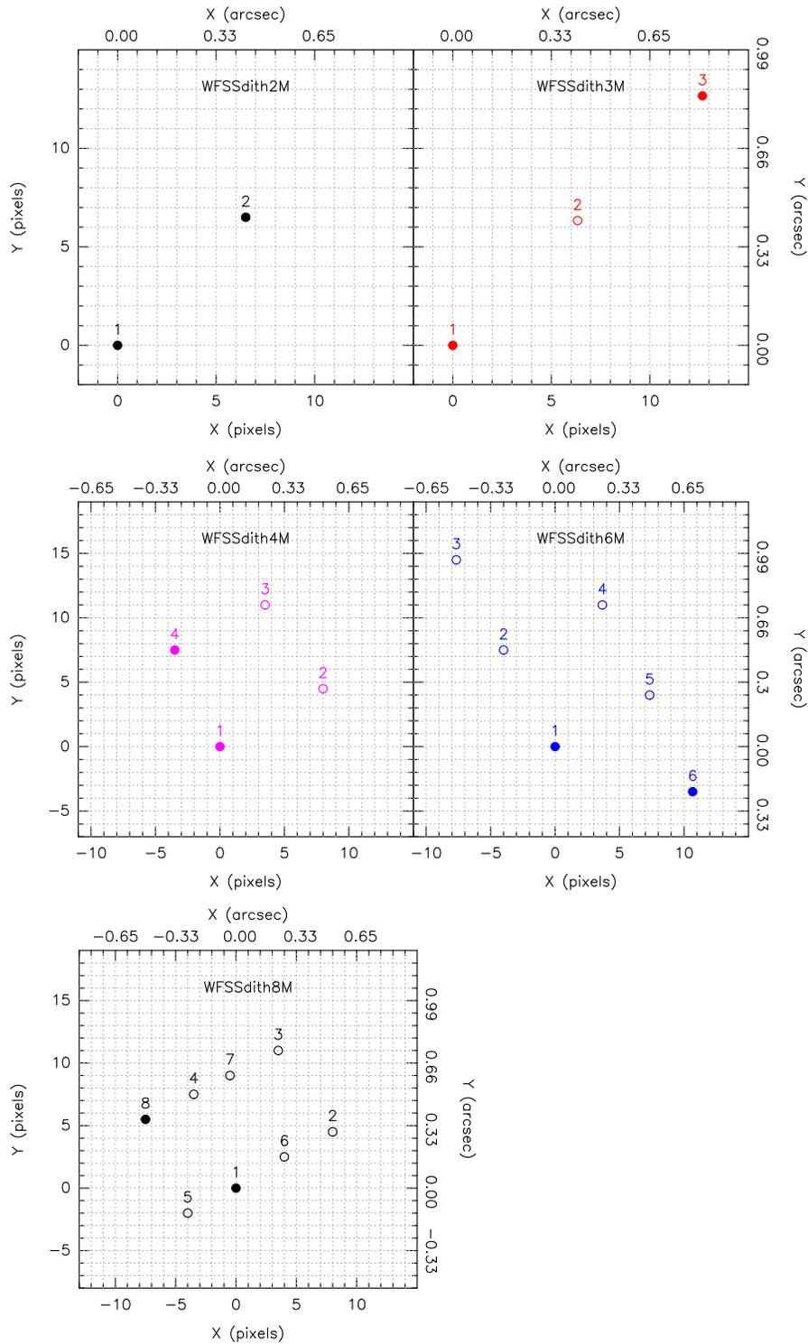
**Figure 4: NIRISS/WFSS “Medium” dither patterns with  $\sim 0.6$  arcsec dither steps. The label above each dither step indicates the step number (cf. Tables A1-A3). Filled circles indicate positions where direct images will be taken in addition to grism images. Preliminary dither pattern names are mentioned near the top center of each panel. The 8-pt dither pattern has smaller steps (see §7.1).**
