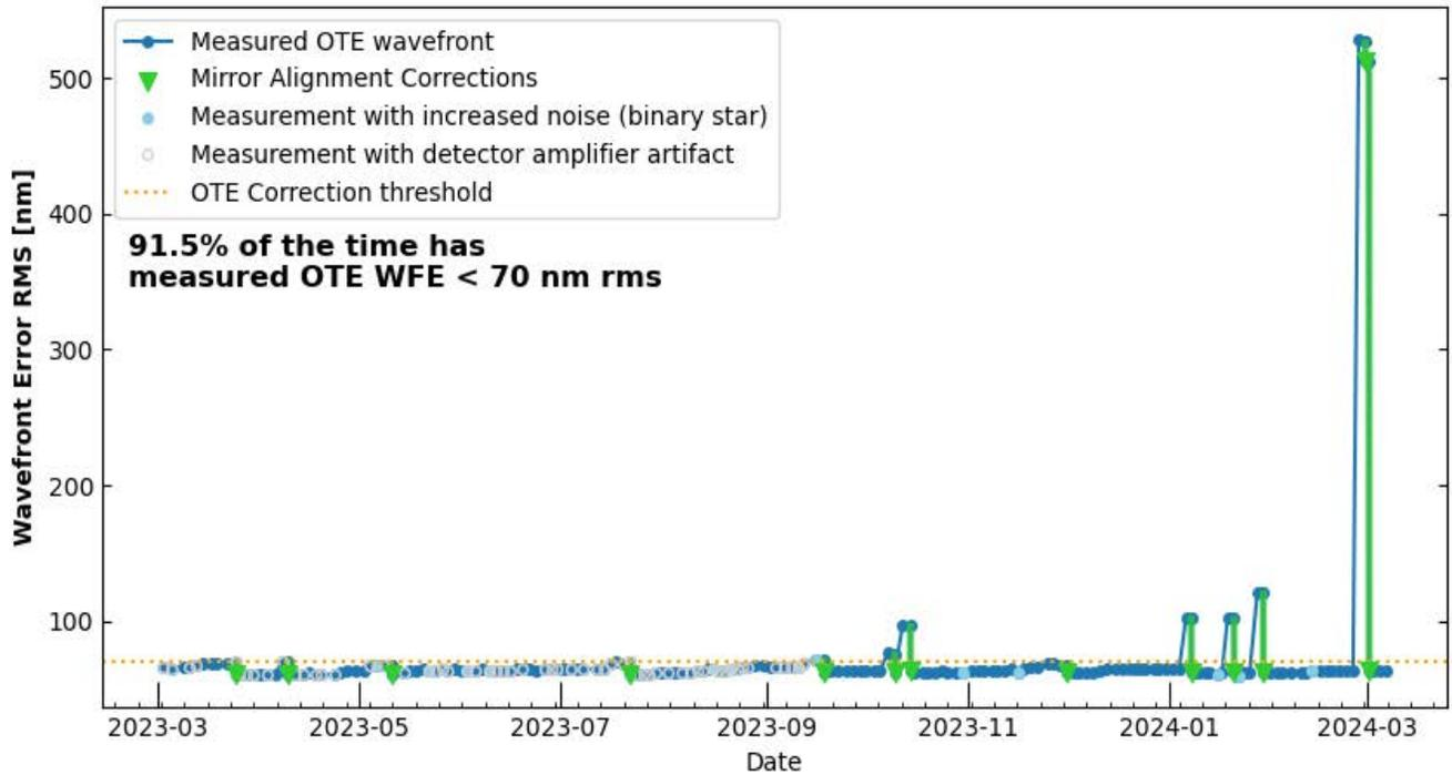
**Figure 1:** Time series of measured telescope root mean square (RMS) wavefront error. The outlier nature of the 2024 Feb event is clear. The observed change in wavefront is many times larger than seen in other events during science operations. The previous largest event was a 240 nm rms mirror move on 2022 July 12, not shown.
