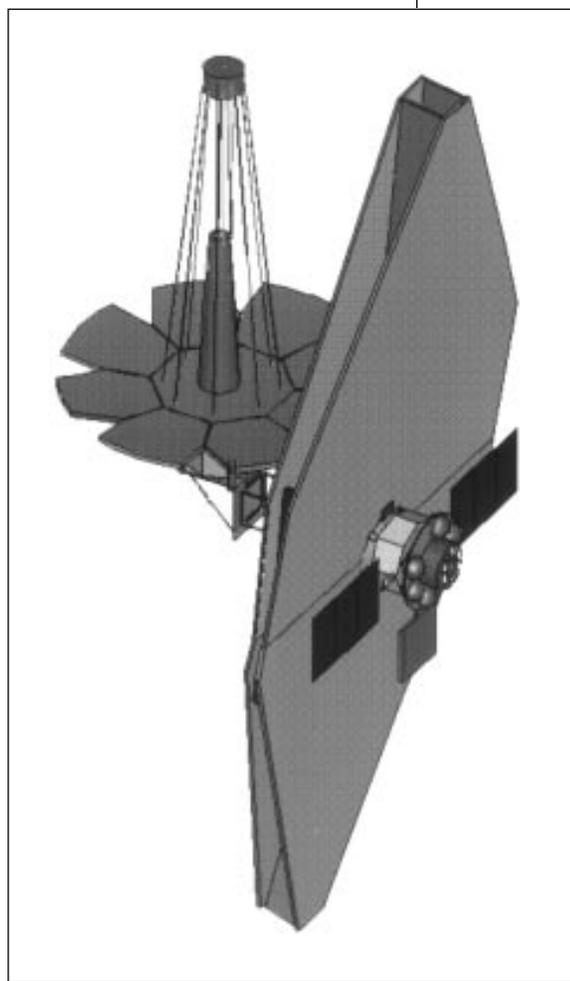
*A design concept for the Next Generation Space Telescope. Shown is the deployed primary and secondary mirrors, the large sunshield with solar arrays and phased array antenna, and a module containing the warm spacecraft electronics and pointing system. The radiatively cooled instrument module is behind the sunshield and below the deployed primary mirror. (GSFC)*
