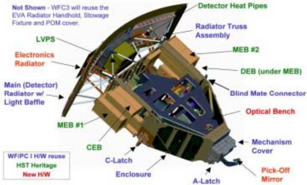
Figure 6. Solid Model of WFC3 showing re-use of components.
