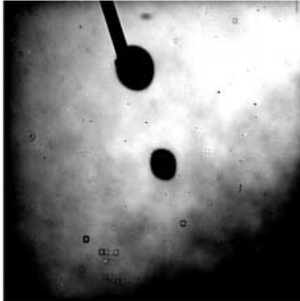
**Figure 3:** Earth flat taken through F330W, displayed between 95% - 105% of the median image value.
