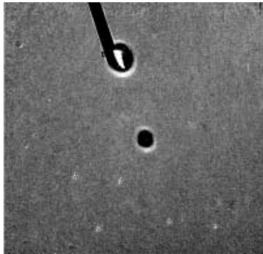
**Figure 6:** Orion Nebula-derived response pattern divided by the F606W coronagraphic LP-flat and the initial F606W spot flat. Differences between the on-orbit spot patterns and those in the prelaunch data result in the 4%-5% residuals seen around the spots. Displayed between 97%-105% of the median image value. Residuals caused by stars are visible.
