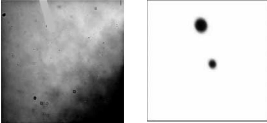
**Figure 5:** (Left) Coronagraphic P-flat for F606W derived from the prelaunch data. The spots have been replaced by regions patched in from the normal F606W flat. Displayed between 95%-105% of the median image value. (Right) Spot flat for F606W derived from the prelaunch flat and including the correction based on the residuals seen in the Orion Nebula-derived response pattern.
