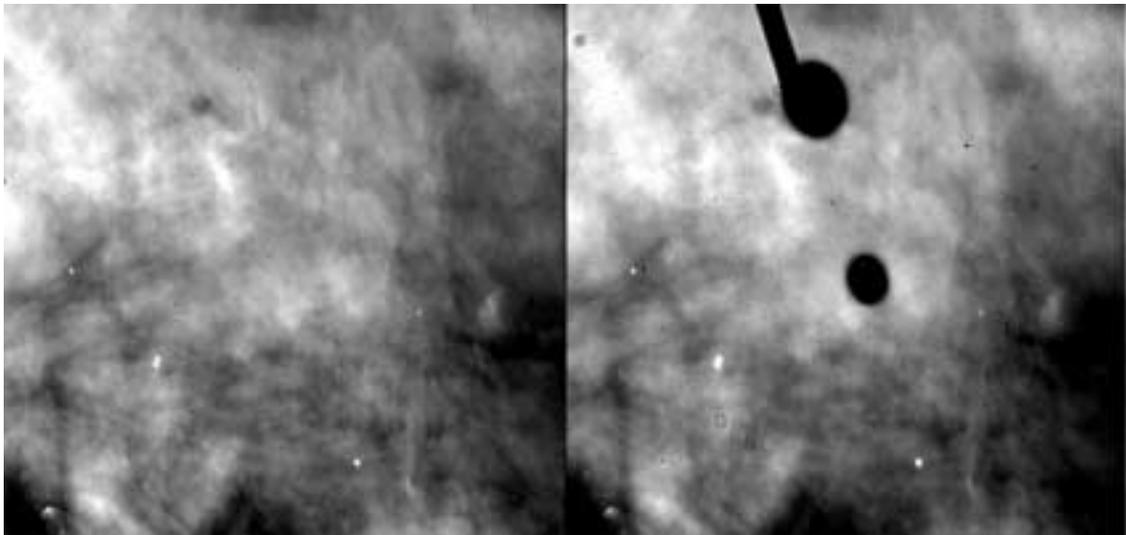
**Figure 1:** (Left) Noncoronagraphic HRC image of a region of the Orion Nebula after flat fielding. The frame is composed of dithered images, so the occulting finger has been filled in. (Right) HRC image of the same region taken with the coronagraph in place and with no flat fielding. Both images are displayed between 80% - 120% of the median image values.
