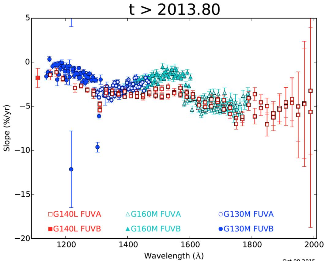
**Figure 2. COS FUV TDS slope during Cycle 22, expressed in percent per year and plotted as a function of wavelength for the different gratings (see legend). FUV A is plotted as open symbols and FUV B as filled symbols. G130M is represented with blue circles, G160M with cyan triangles, and G140L with red squares. The variation in trend from segment to segment within a grating is apparent.**
