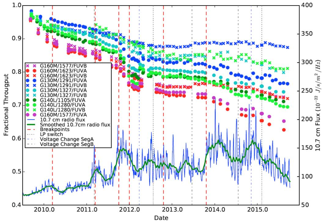
**Figure 1. Decline of the COS FUV spectroscopic sensitivity over time (symbols, see legend) compared to the solar activity** directed at Earth as tracked by the 10.7 cm flux (blue solid line original data; green solid line smoothed data). The dashed red vertical lines represent breakpoints in the piece-wise function used to model the TDS. The dotted grey vertical lines mark the LP move, and the dot-dashed grey vertical line corresponds to change in operational voltage.
