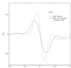
The FGS has been used successfully to determine the angular diameters of non-point sources. The example given in the figure at left shows the Transfer Function of a Mira-type variable (Lattanzi *et al.* 1997) superposed on the S-Curve of a point source. The extended source - a disk of  $78 \pm 2$  mas - is clearly distinguishable from a point source.
