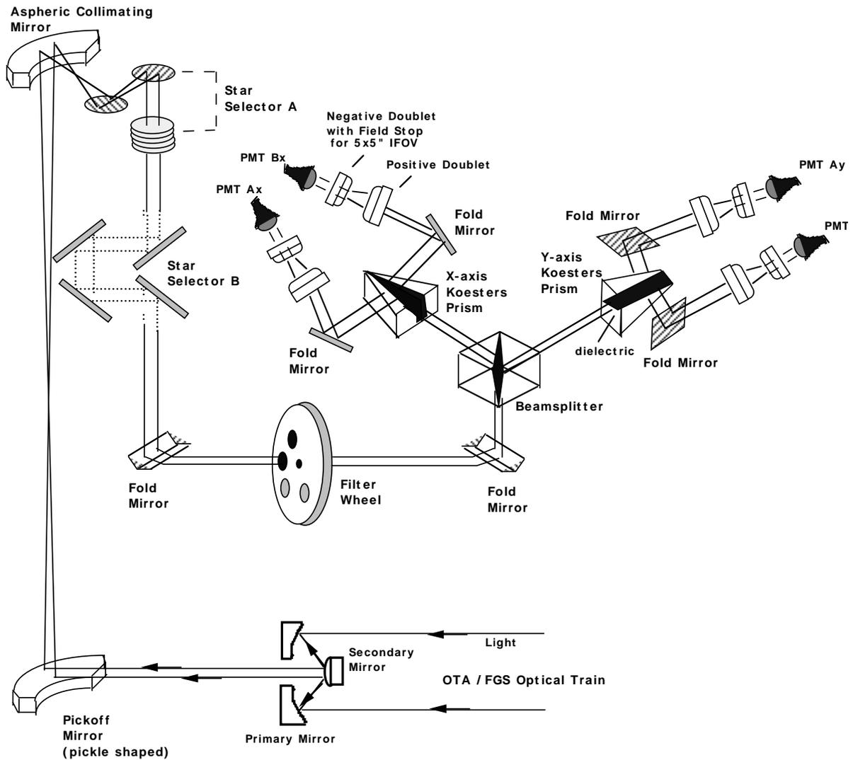
For the FGS to sense angular displacements in the plane of the prism's dielectric surface, another, orthogonally aligned Koesters prism is required. This prism intercepts the other beam emitted by the polarizing beam splitter.
