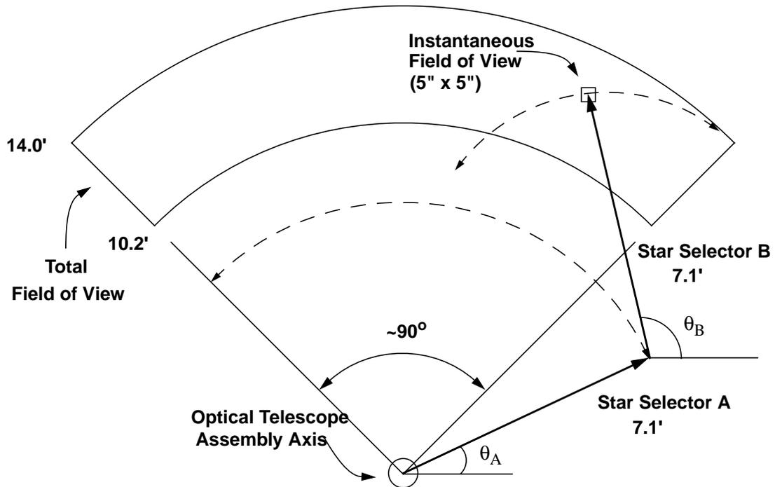
After exiting the SSA, the beam passes through a field stop which minimizes scattered light and narrows the IFOV. The beam next encounters the Star Selector Servo B assembly (SSB), which consists of a rigid assembly of four mirrors which, like SSA, can be rotated about an axis which is parallel to HST's optical axis. Upon exiting the SSB assembly, the beam encounters a fold flat mirror, the filter wheel assembly, another fold flat mirror, and finally the polarizing beam splitter.
