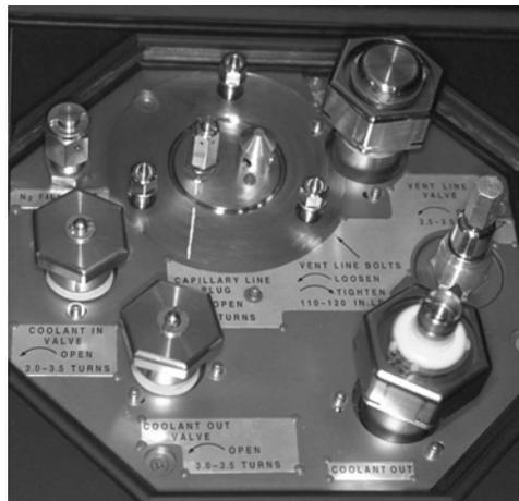
Figure 2 – Plumbing Interface Plate
