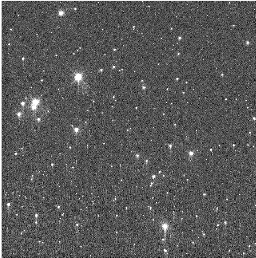
Figure 9.: The CTE loss can be seen in this image (obmj01050) as the flux trails underneath the sources. For STIS, the most significant CTE loss is in the Y direction, called parallel CTE (Van Dyke Dixon, 2011). The amplifier is located at the top of the detector and the trails are caused by a delay in the release of charge during readout.
