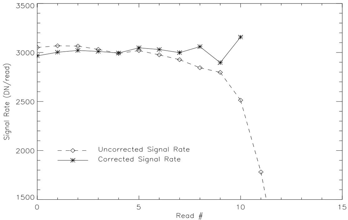
**Figure 3:** Corrected and uncorrected signal rates for pixel (400,400) in one of the three ramps used to calculate the correction coefficients. A perfectly linear detector would have a constant signal rate, and therefore a horizontal line in this plot. The corrected signal rates extend only to read 11 because the signal reached saturation at this point.
