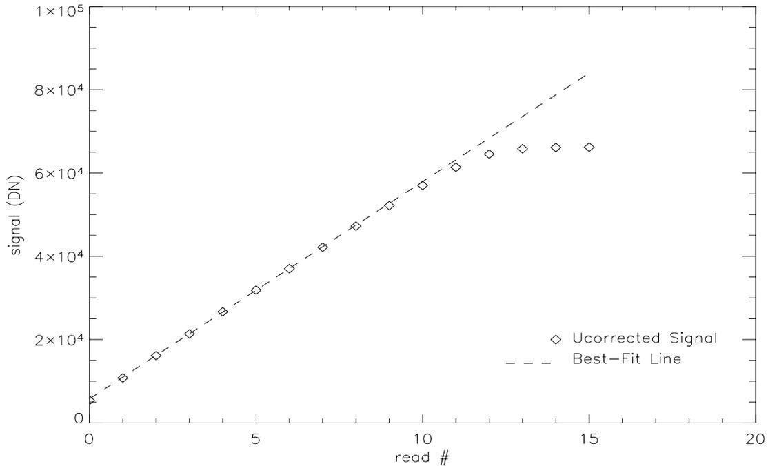
**Figure 1:** Signal measured in the original ramp (diamonds) versus read number within the ramp, for pixel (400,400). The best-fit line from a fit to reads 3 through 6 is plotted as the dashed line. The saturation level, where the measured signal deviates from the best-fit line by 5%, is calculated to be 63,840 DN.
