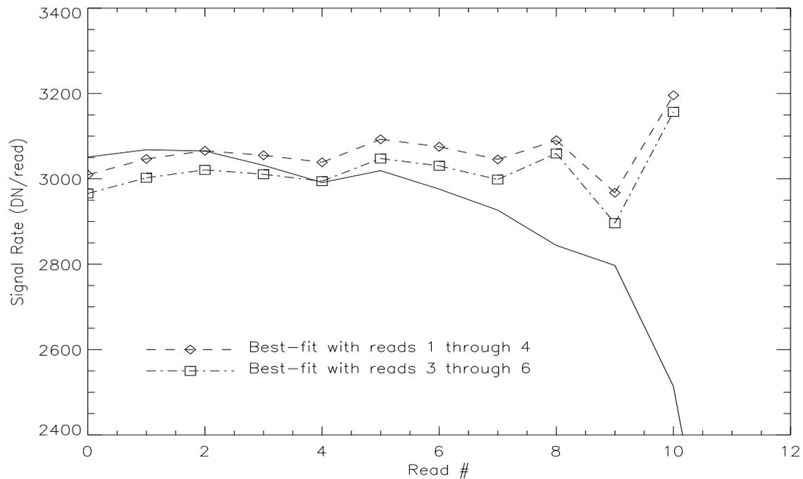
**Figure 5:** Same plot as Figure 3, with signal rates before and after different non-linearity corrections. Squares show the same correction as in Figure 3. Traingles show the signal rate with correction coefficients based on best-fits to reads 1 through 4 , rather than reads 3 through 6.
