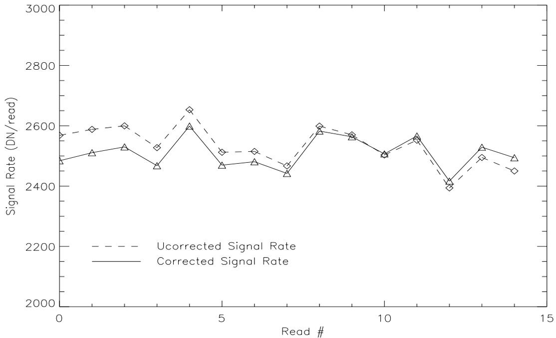
**Figure 4:** Corrected versus uncorrected signal rates for pixel (400,400) in gain data taken independently from the linearity data shown in Figures 1 through 3. The correction here is more subtle, but still shifts a ramp with an overall decreasing signal rate to one with a constant signal rate.
