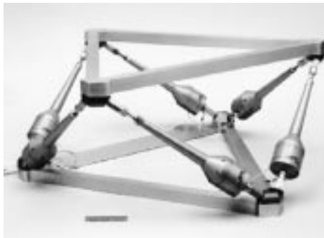
FIGURE 10.7. A hexapod vibration-suppression stage using active and passive members. (NASA/JPL)
