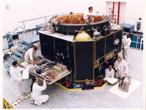
Figure 3. Extensive use of composite materials helped cut mass from 32,000 to 10,110 lb.
