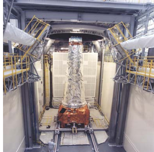
Figure 7. Chandra at NGST Thermal Vacuum Chamber
