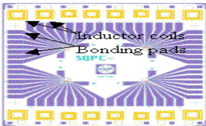
Figure 6. 8x10 mm substrate for SETs and submillimeter detectors. Chip has 16 rf tank circuits.
