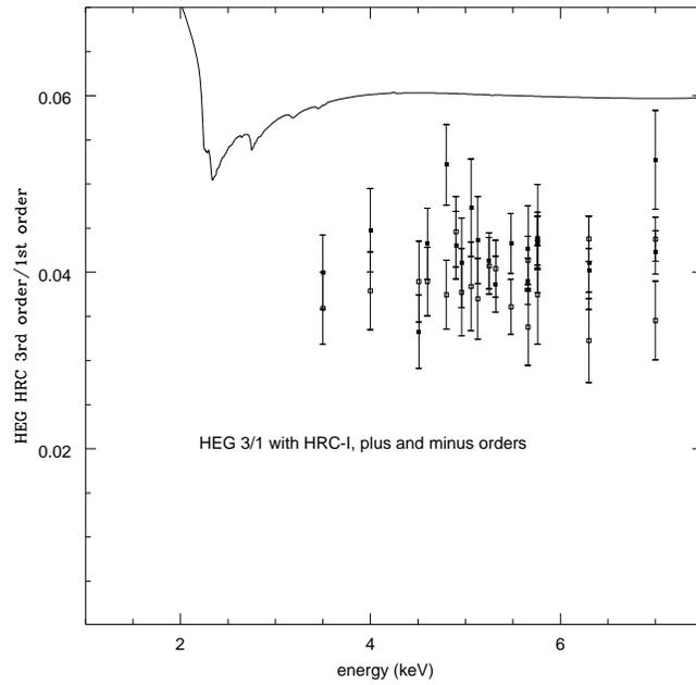
**Figure 4.** Measured HEG ratios for 2nd,3rd, and 4th orders with HRC-I. The solid curve represents the predicted ratios. Hollow points indicate ratios of negative orders, and solid points refer to positive orders. The error bars are due to counting statistics. The measurements systematically fall below predictions.
