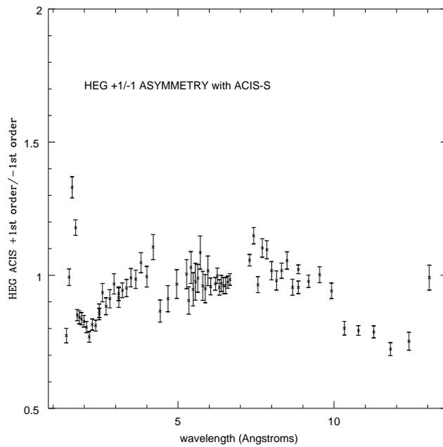
**Figure 6.** Ratio of +1 to -1 for HEG grating on ACIS-S. Structure is due to detector effects.
