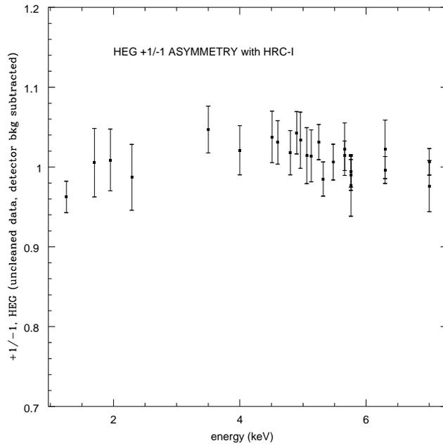
**Figure 2.** Ratio of +1 to -1 for HEG grating on HRC-I. In general, departures from unity are expected to be caused by intrinsic grating asymmetry, detector nonuniformity or bias angle effects.
