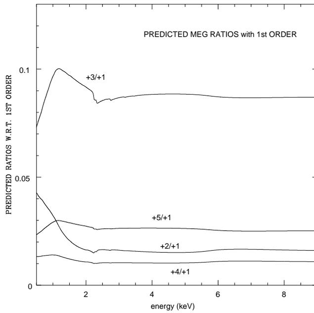
**Figure 3.** Expected ratios of orders 2 through 5 with respect to 1st order for HEG (top) and MEG (bottom). These are based on subassembly calibrations.
