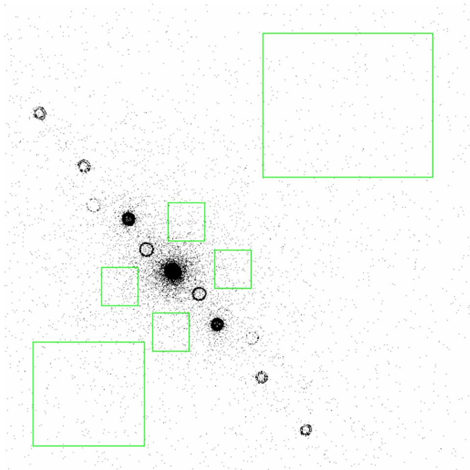
**Figure 1.** HETG + HRC-I test at 7 keV. Positive orders are dispersed toward the upper left in the figure. The large box, top right, is used to estimate detector background. The small boxes around zero order sample mirror-scattered events. The data have been “cleaned” to remove saturated events.
