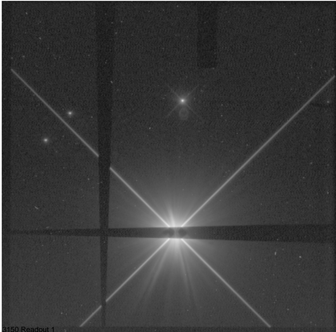
Figure 1. A clear-CCD-mode image of the HST standard star HD60753 positioned to intercept a coronagraph bar, from SMOV program 7088. The square field is 50 arcsec across; the large rectangular bar is 3 arcsec by 10 arcsec; the tapered bars are from 0.5 arcsec to 3 arcsec in width (1.8 arcsec at HD60753's location); and the crooked bar is 0.5 arcsec wide. The exposure duration is 1800 sec.
