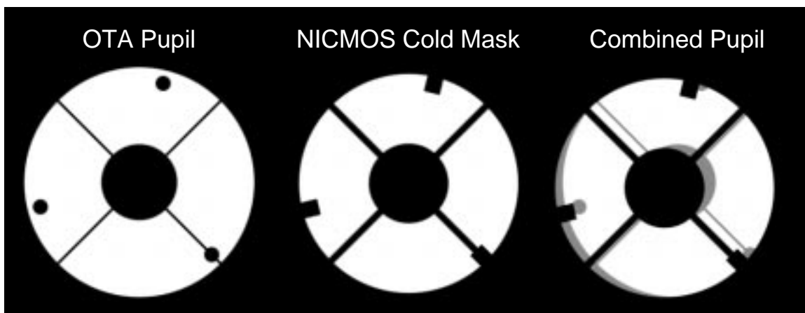
Figure 3. Simulated obscuration patterns for HST and NICMOS. On the left is the telescope pattern with secondary mirror obscuration, spiders, and mirror support pads. The middle image shows the NICMOS 2 cold mask, which would optimally be aligned with the telescope obscurations. On the right is the predicted NICMOS 2 obscuration pattern with the cold mask shifted. The telescope obscurations are color coded grey.
