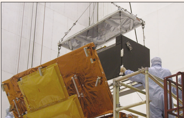
ACS being lowered into the SIPE.
