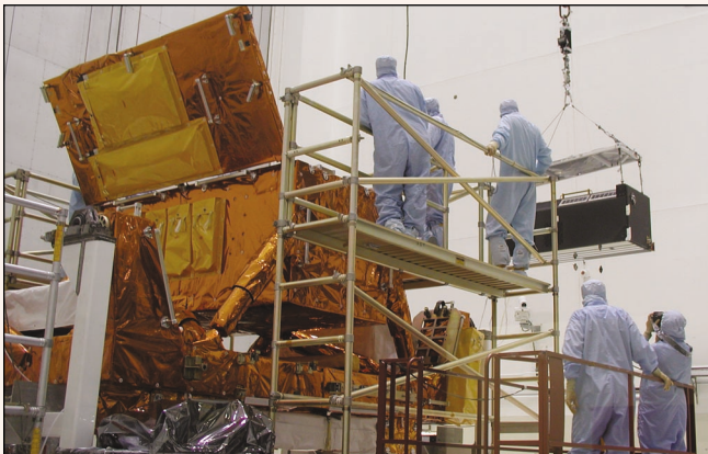
The SIPE (Science Instrument Protective Enclosure) waiting for ACS to be installed.
