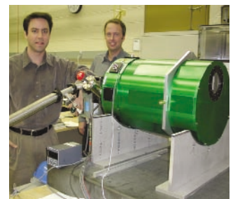
Figure 4: Testing dewar in IDTL lab. Don Figer (left) and Bernie Rauscher (right) showing the new dewar in the Independent Detector Testing Laboratory at JHU/STScI that will be used to test and characterize competing detector technologies for the NGST.
