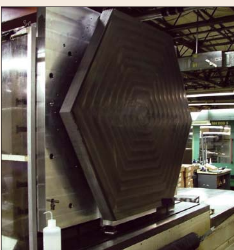
Figure 1: The primary mirror segment of the JWST Engineering Demonstration Unit, mounted for machining at Axys Technologies.
