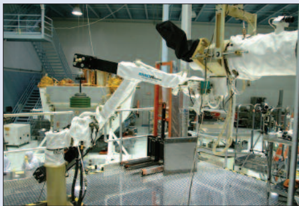
Figure 2: The MD Robotics 1-g test bed for Dextre, shown deployed in the cleanroom at the Goddard Space Flight Center. The test bed is a fully functional, high fidelity representation of one of the two Dextre arms.
