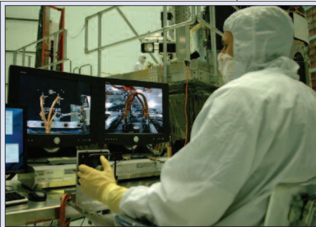
Figure 5: An operator in the Goddard clean room controlling Dextre with a joystick. Actual operations will entail a combination of joystick control and pre-programmed, computer-driven operations, initiated by the operator with “go/no-go” commands.
