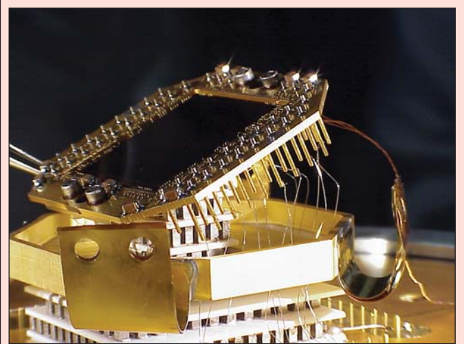
Figure 1: Infrared focal plane mounted on its six-stage thermal electric cooler, prior to installation of the cold baffle. Image courtesy of Ball Aerospace.
