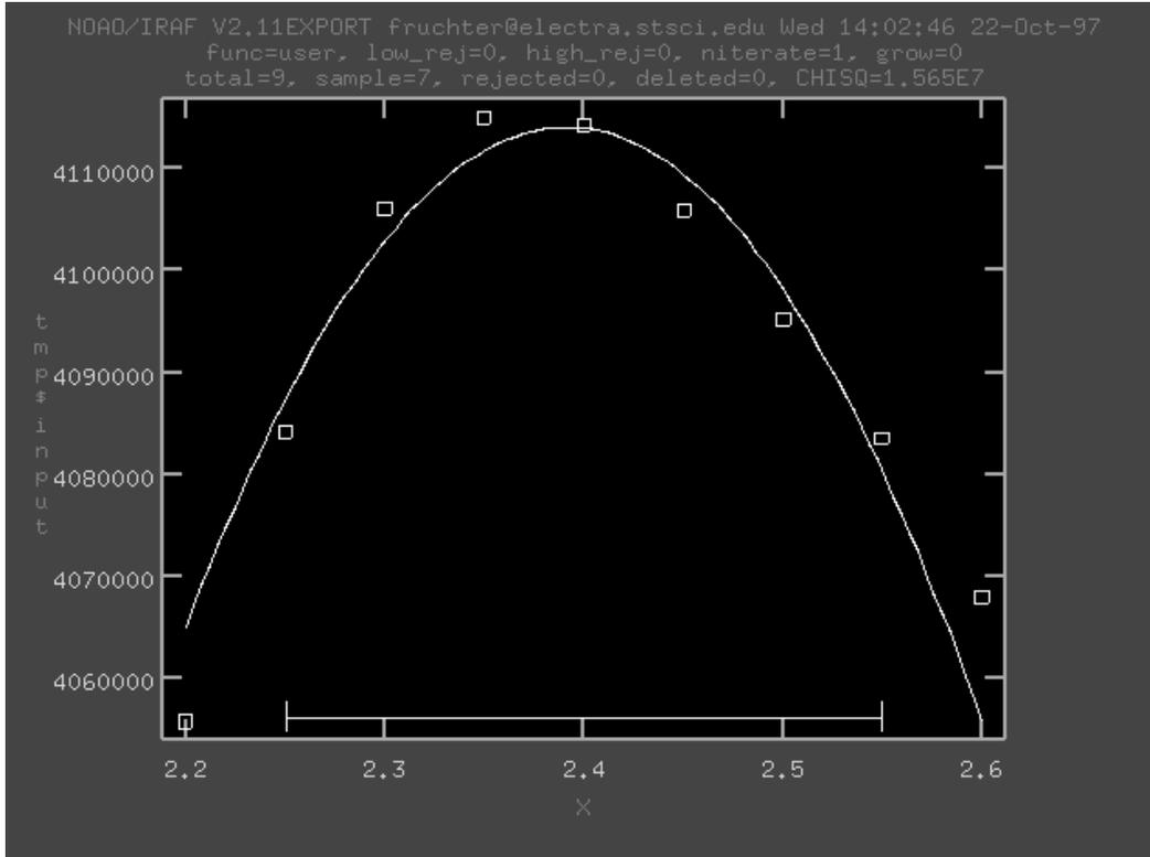
Figure 6. The graphical output of the task `rotfind`, used in this case two determine the rotation angle between two WFPC2 images of GRB 970228. According to the header, the change in orientation between these two images was 2.4 degrees. An error of 0.01 degrees is typical in measuring the rotation between two WFPC images.
