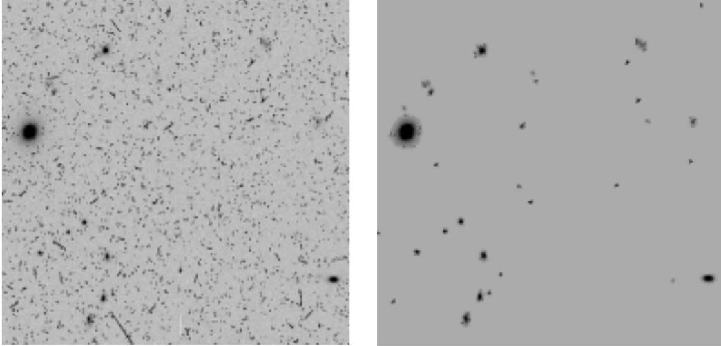
Figure 5. A comparison of a raw image and the output image from `precor`. The sky is set to zero, while true objects are preserved. As a result, essentially all cosmic rays, with the exception of those on top of detectable astronomical objects, are removed.
