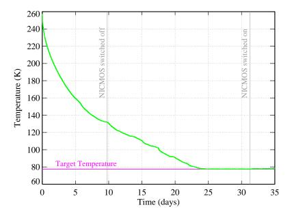
Figure 1. Time line of the NICMOS detector cool down.
