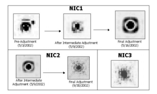
Figure 3. NIC1 and NIC2 PSFs before and after PAM tilt correction for coma. NIC3 PSF is shown for comparison.
