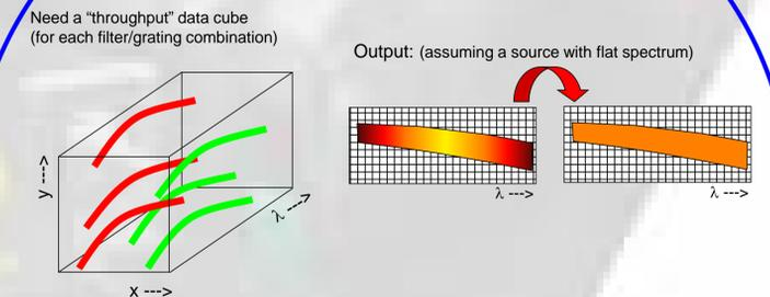
Goal: to correct for the total instrumental throughput variations, both as a function of wavelength (e.g. optics transmission, blaze function) and field angle (e.g. DQE, vignetting).
