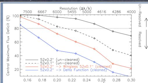
Figure 3: Simulation statistics (see Figure 2) allow us to calculate the relative resolutions of the G140M 52x0.1" and 52x0.2" apertures (solid and dashed lines) compared to spectral cleanings performed on simulated STIS/G140M/52x0.2" data. Our delta-function and 'wingless' 52x0.1" "cleanings" of input+52x0.2" simulations achieve "70%" and "50%" higher spectral resolution than the input+52x0.2" and input+52x0.1" simulations, respectively.
