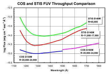
The figures above and below compare COS Primary Science Aperture (PSA) and STIS medium resolution (M mode) performance by indicating the limiting flux for which S/N=10<sup>†</sup> can be achieved in 3600 sec exposures with uniform binning corresponding to R~10,000 (bins of 0.15 Å for FUV and 0.24 Å for NUV. The superior light gathering power of COS provides >10x the FUV throughput of STIS and up to 70x STIS FUV observing speed.
