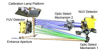
External light enters at lower left; common path to first element at lower right. FUV path in green; NUV path in blue; PtNe and  $D_2$  input calibration beams in tan.
