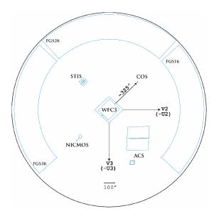
The HST focal plane showing the instrument complement after Servicing Mission 4. The COS FUV and NUV channels view the same 2.5 arcsec patch of sky, but not simultaneously. Instrument apertures and separations are shown to scale.
