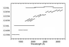
Wavelength coverages available with common COS spectroscopic modes. The ranges for different grating tilts are offset in the vertical direction. Additional settings may be available for some modes. Notice noncontinuous spectral ranges for NUV modes.
