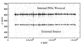
The figure above shows the typical spectrum format for a single COS FUV MCP detector segment. The COS FUV detector consists of two such segments separated by a small gap. Two spectra may be recorded as shown above. The lower spectrum is from an external source illuminating the prime science aperture (PSA); the upper spectrum is from the internal PtNe wavelength calibration lamp which illuminates the wavelength calibration aperture (WCA).
