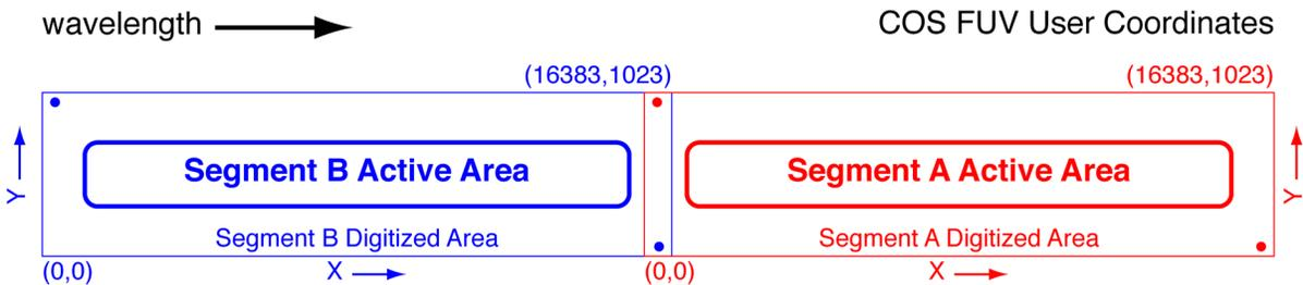
This diagram is drawn to scale, and the slight curvature at the corners is also present on the masks of the flight detectors. Wavelength increases in the direction of the increasing X coordinate. The red and blue dots show the approximate locations of the stim pulses. The numbers in parentheses show the pixel coordinates at the corner of the segment's digitized area; the two digitized areas overlap in the region of the inter-segment gap.
