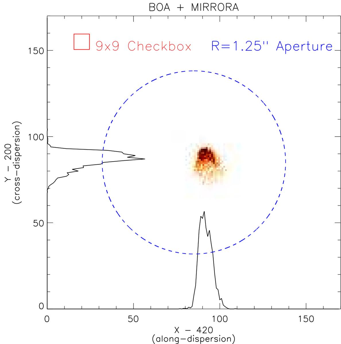
NUV image of a point source observed through the BOA aperture using MIRRORA. The limits of the plot represent the  $170 \times 170$  pixel image discussed in Section 8.3.3. Also shown are the COS aperture (blue circle of radius  $1.25''$ ) and the  $9 \times 9$  checkbox used by ACQ/SEARCH. The dispersion and cross-dispersion axes show the one-dimensional light distributions on this un-centered target. This pointing is typical of that expected after an ACQ/SEARCH, but before additional peak-ups.
