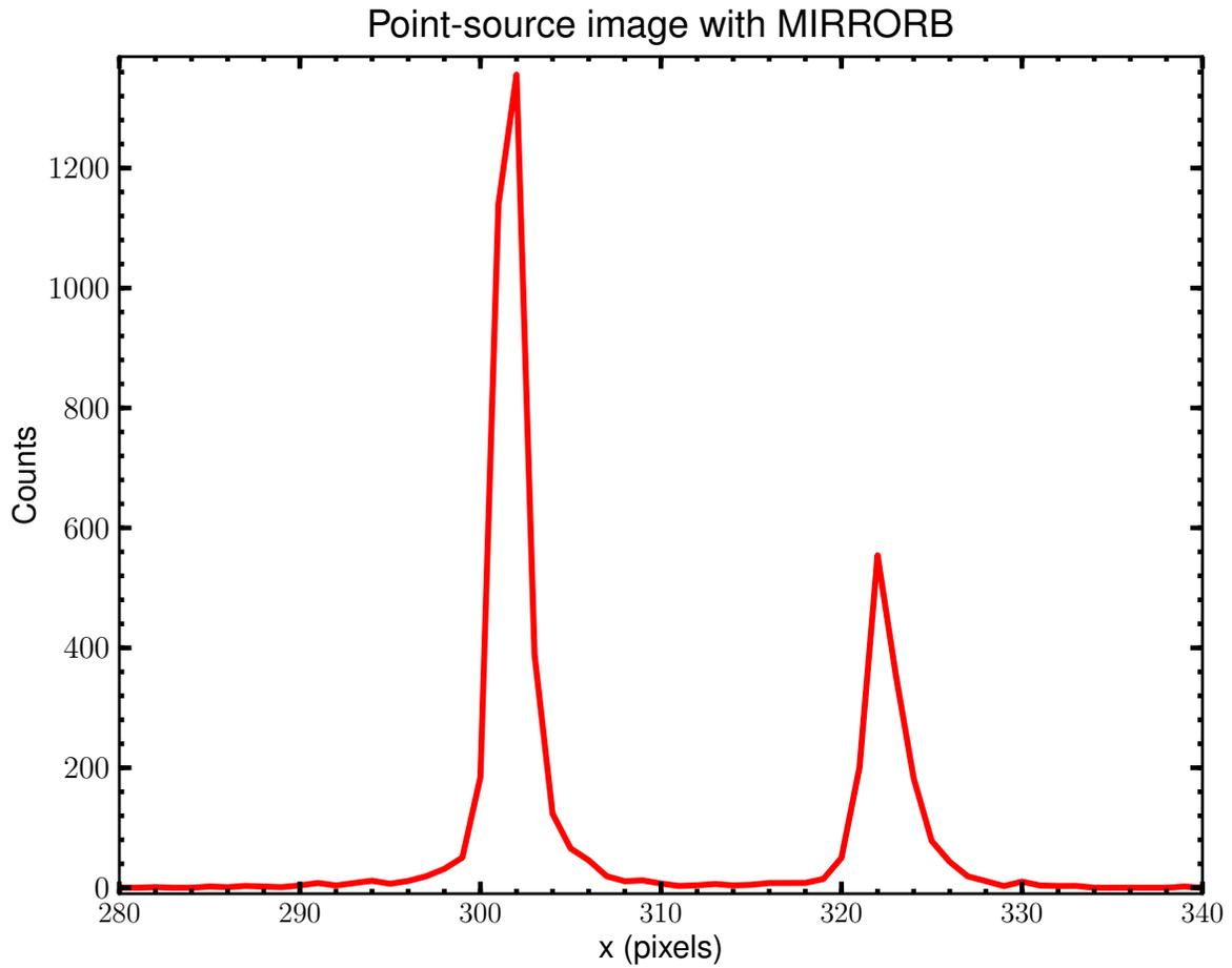
Cross section through the center of an image obtained with the PSA and MIRRORB. The secondary peak has an amplitude about half that of the primary peak and is displaced by 20 pixels (center to center) in the  $x$  (dispersion) direction.
