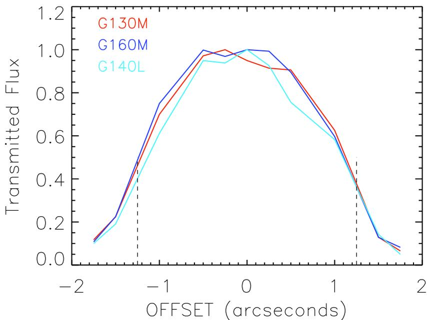
Transmitted flux as a function of displacement from aperture center in the cross-dispersion direction for all three FUV gratings. The dotted lines mark the edge of the aperture ( $1.25''$ ). For all gratings, the absolute transmission for a centered point source is at least 95%.
