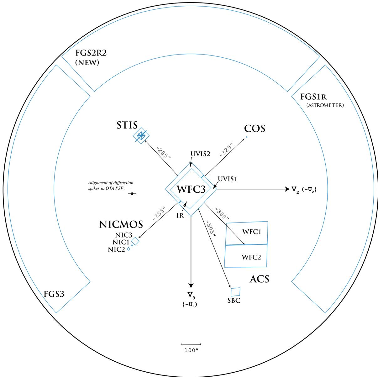
This drawing shows the entire *HST* focal plane and the apertures of the scientific instruments. The view is from the rear of the telescope looking forward toward the sky, the opposite of the sense of [Figure 3.2](#).
