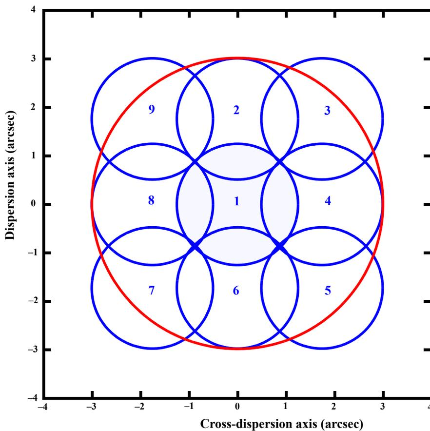
This example was executed with the default STEP-SIZE of 1.767 arcsec. The blue circles represent the nine positions of the aperture, each 2.5 arcsec in diameter, and the numbers show the sequence of steps. The large outer circle in red has a radius of  $\sim 3$  arcsec. An initial pointing that was good to 1 arcsec ( $1\sigma$ ) would result in a successful acquisition with a  $3 \times 3$  pattern 99.5% of the time.
