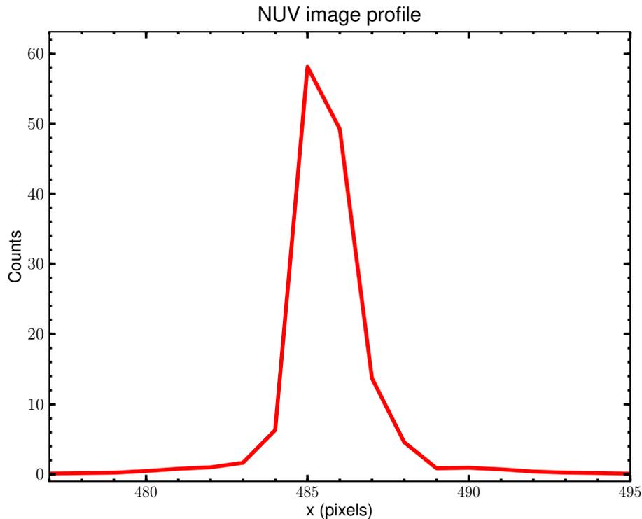
Profile through COS imaging PSF in the  $x$  direction. The red solid line represents a slice through the central row of the profile.
