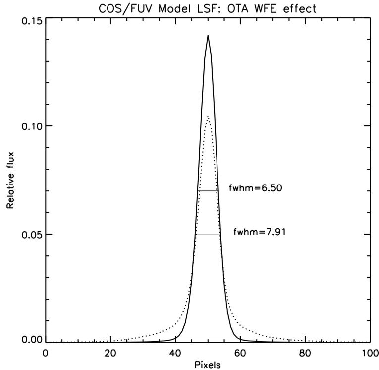
Model LSFs for G130M at  $1309 \text{ \AA}$ , normalized to a sum of unity. The solid line represents a model LSF that incorporates the spherical aberration of the OTA; it is well-fit by a Gaussian with FWHM = 6.5 pixels. The dotted line represents a model that also includes the HST mid-frequency wave-front errors. It shows a larger FWHM and broad, non-Gaussian wings.
