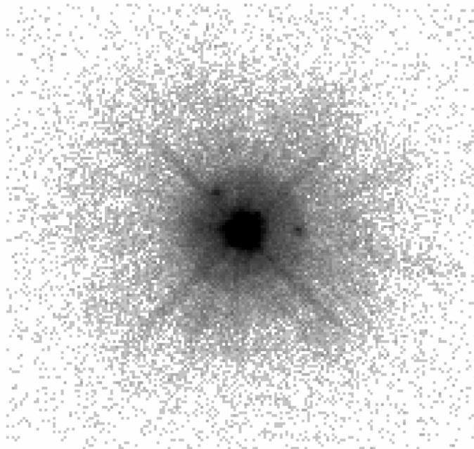
Negative greyscale rendering of a deep COS NUV image of a point source. This figure is plotted with a logarithmic intensity scale and covers about 6.5 arcsec along each axis. Note the two ghost images to the right and upper left of the center of the PSF.
