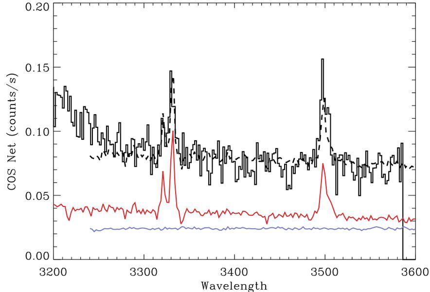
Black curve is stripe B of the G230L CENWAVE = 3360 spectrum of NGC 6833. Blue curve is an FOS spectrum of NGC 6833 over the same wavelength range (units are Ångstroms). Red curve is an FOS spectrum of the 1600 - 1800 Å region, plotted as  $f(2\lambda)$ . The FOS spectra have been rescaled by arbitrary amounts for display purposes. The dashed curve, a combination of the two FOS spectra, reasonably reproduces the COS spectrum.
