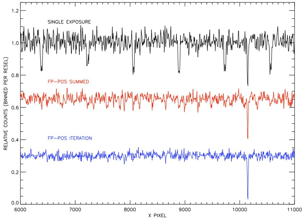
On-orbit FUV observations of a white dwarf. The black curve represents a single exposure. The red curve represents the sum of spectra taken at several FP-POS settings. The blue curve represents the sum of spectra taken at several FP-POS settings, each flat-fielded before being combined.
