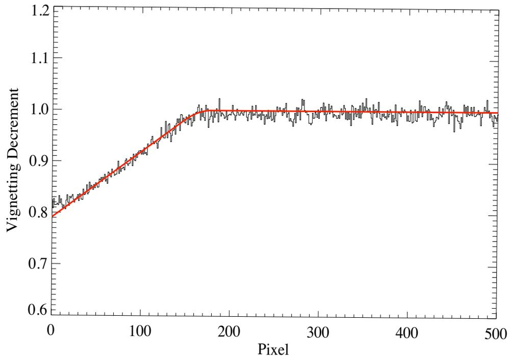
Vignetting profile of the medium-resolution gratings as a function of pixel location showing the linear decrease in throughput near the low-pixel edge of the NUV detector. The red line shows the best fit to the profile obtained from observations of the white dwarf G191-B2B.
