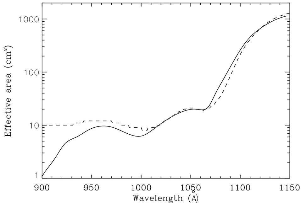
Segment B effective area of the COS G140L grating at wavelengths between 900 and 1150 Å. Dashed line is from McCandliss et al (2009); solid line is from SMOV calibration observations.
