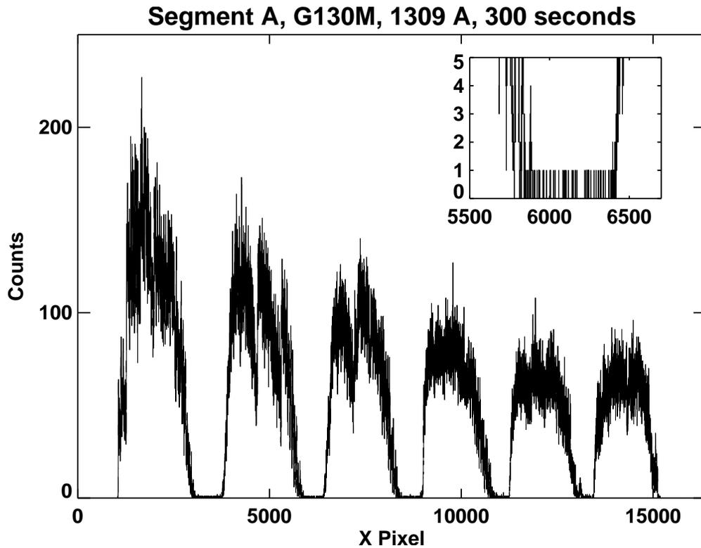
A test exposure obtained during ground calibration using a CO absorption cell. The inset shows an enlargement of the bottom of one of the absorption troughs.
