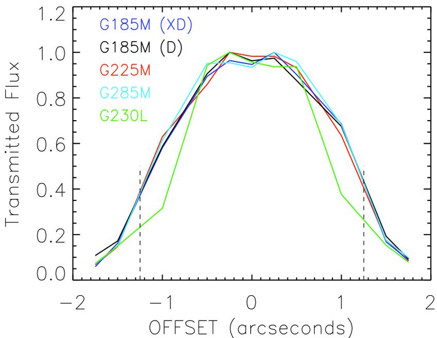
Transmitted flux as a function of displacement from aperture center for all four NUV gratings. The dotted lines mark the edge of the aperture ( $1.25''$ ). The two curves labeled D and XD refer to offsets along the dispersion and cross-dispersion axes, respectively. The other curves trace offsets in the cross-dispersion direction. For all gratings, the absolute transmission for a centered point source is at least 95%.
