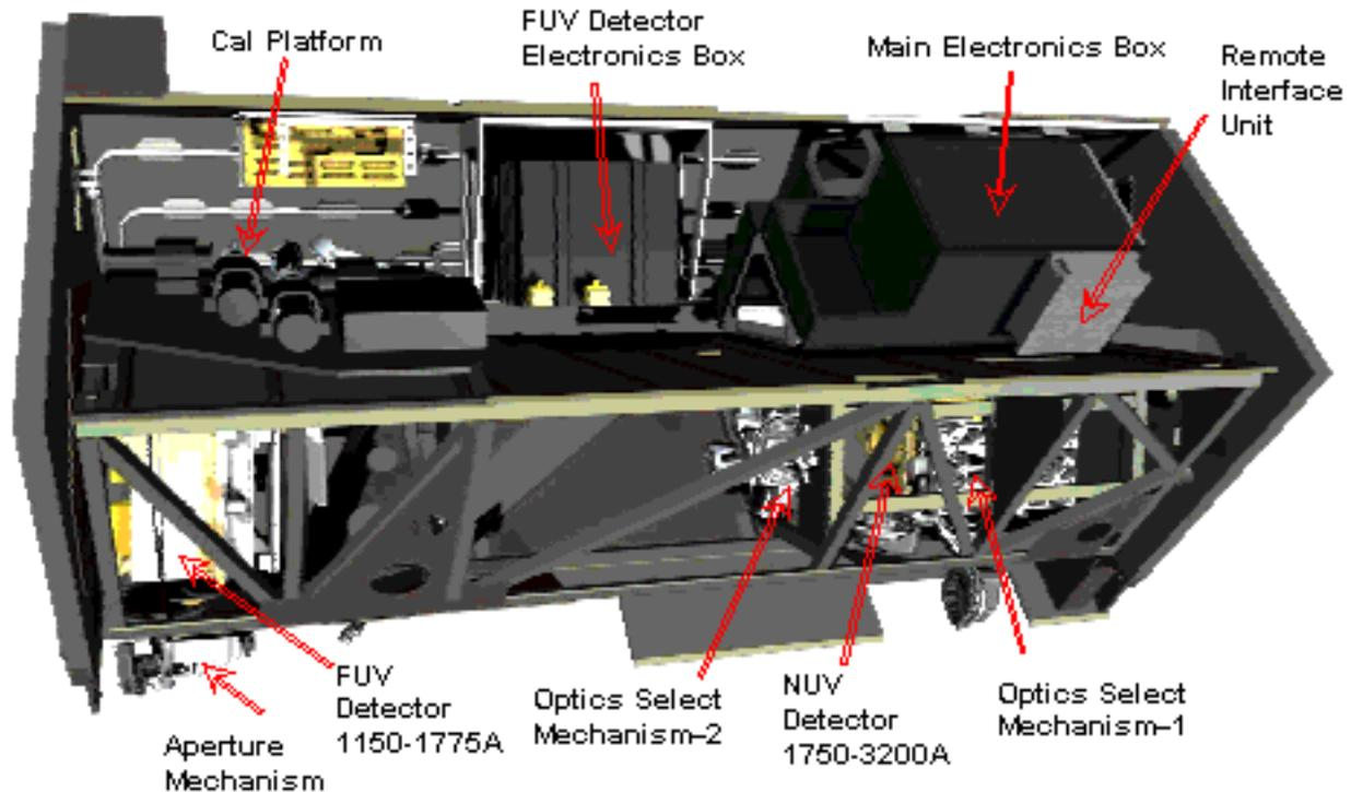
(CAD drawing courtesy of Ball Aerospace.)
