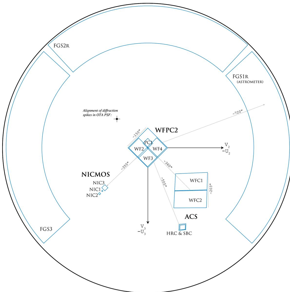
Figure 2.2 shows the layout of the instrument entrance apertures in the telescope focal plane as projected onto the sky.
