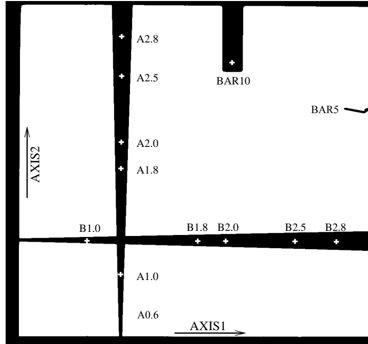
Figure 12.6: Design of the STIS Coronagraphic Mask
