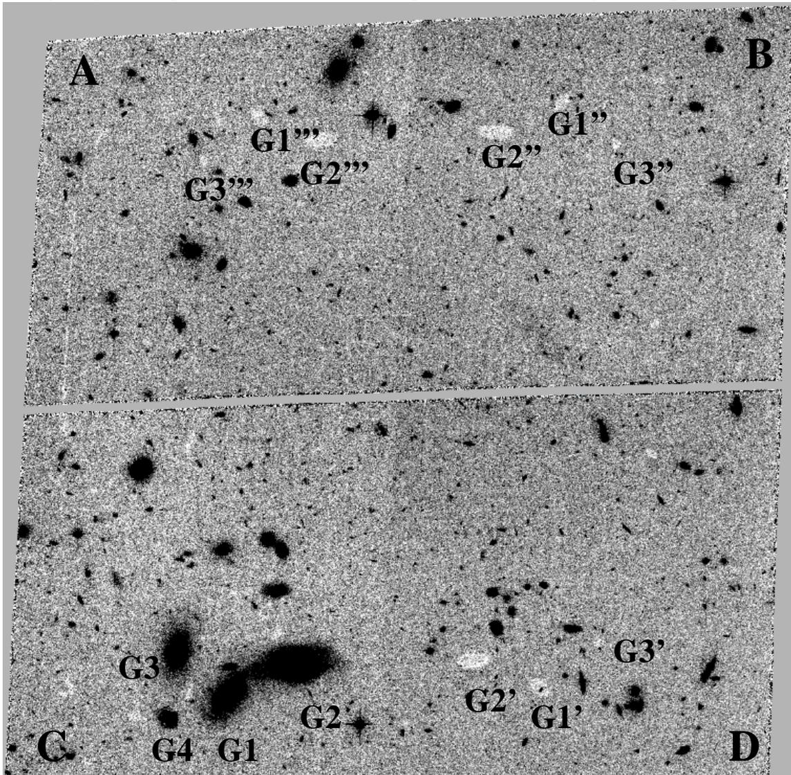
**Figure 2:** Two exposures through the same filter (F606W) and with the same exposure time (22.5 sec), one acquired with GAIN=1 (top) and the second with GAIN=2 (bottom). Each image comprises quadrant C (left half of the image) and quadrant D (right half of the image) abutted together. Cross talk ghost images are observed in the GAIN=1 image, but not in the GAIN=2 one (green arrows point at sources, red ones point at ghosts).
