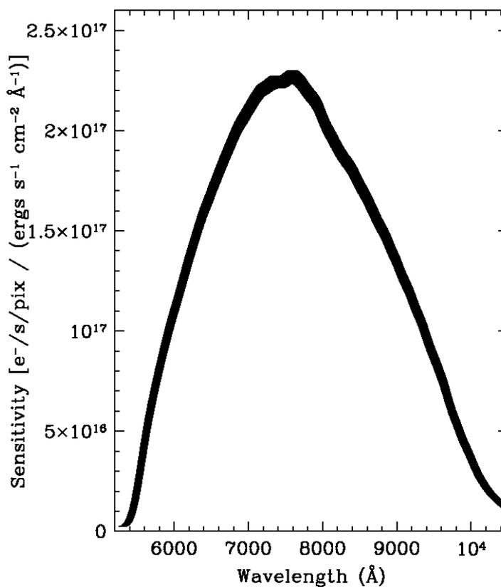
**Figure 8:** The derived sensitivity file in units of electrons per second per pixel for the WFC based on G191B2B at position W0 of CHIP1. The line is broadened by the error bars.
