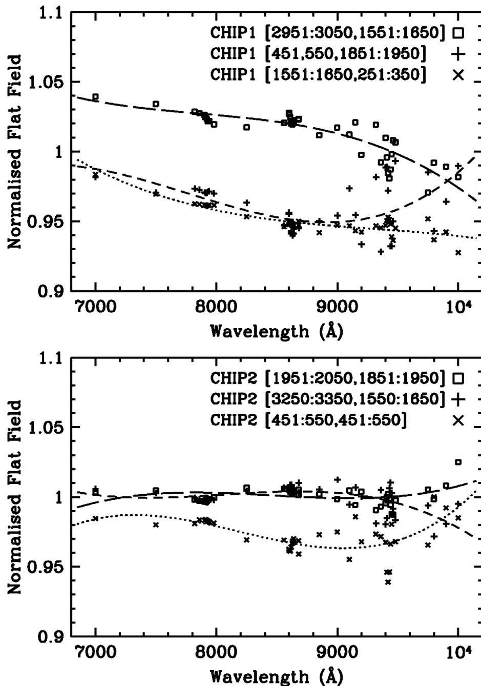
**Figure 1:** The normalised flat-field values, for the ground calibration data, measured in square apertures over the WFC, are plotted as a function of wavelength. The flat-field values correspond to regions which are listed in the figure for each chip (using different symbols) with Chip 1 at the top and Chip 2 below. 3rd order polynomial fits to the points are shown.
