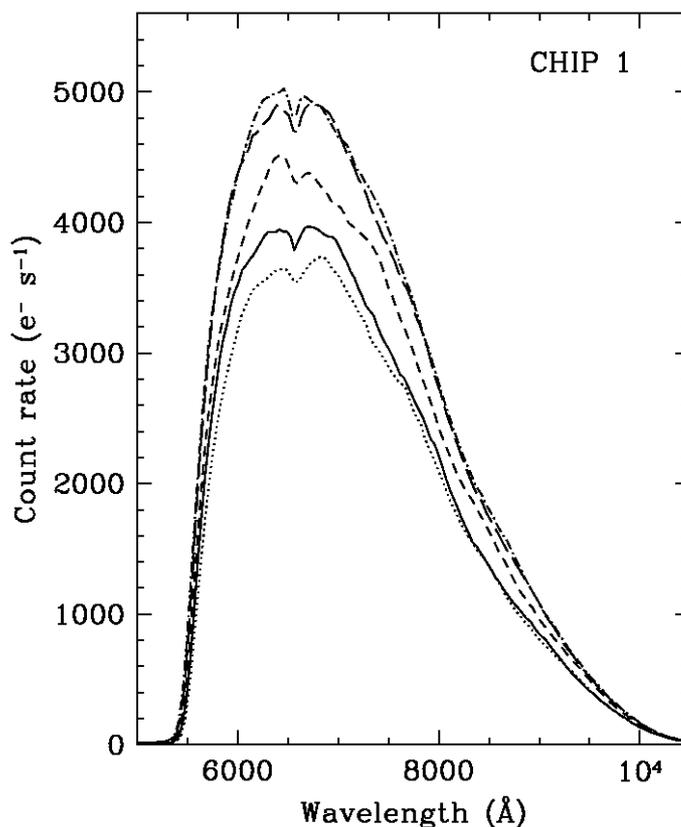
**Figure 7:** Extracted spectra of G191B2B in units of e/s v. wavelength at five positions over WFC CHIP1 are shown, where no corrected flat-field was applied in the extraction process (see text).
