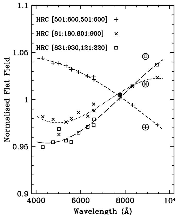
**Figure 4:** The mean values in square apertures of the in-orbit flat-fields for the HRC, are plotted as a function of wavelength. The flat-field values correspond to regions which are listed in the figure and 3rd order polynomial fits are shown by lines. The circled points are for the F892N filter which suffers the most from the effects of detector fringing.
