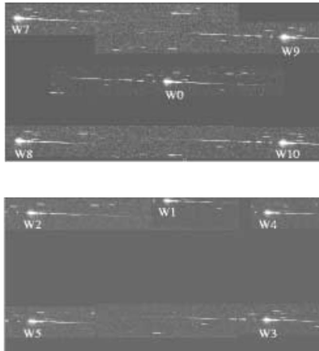
**Figure 6:** Mosaic image of the ten WFC sub-array observations of G191B2B taken with the G800L grism is shown. CHIP1 is upper; CHIP2 lower.
