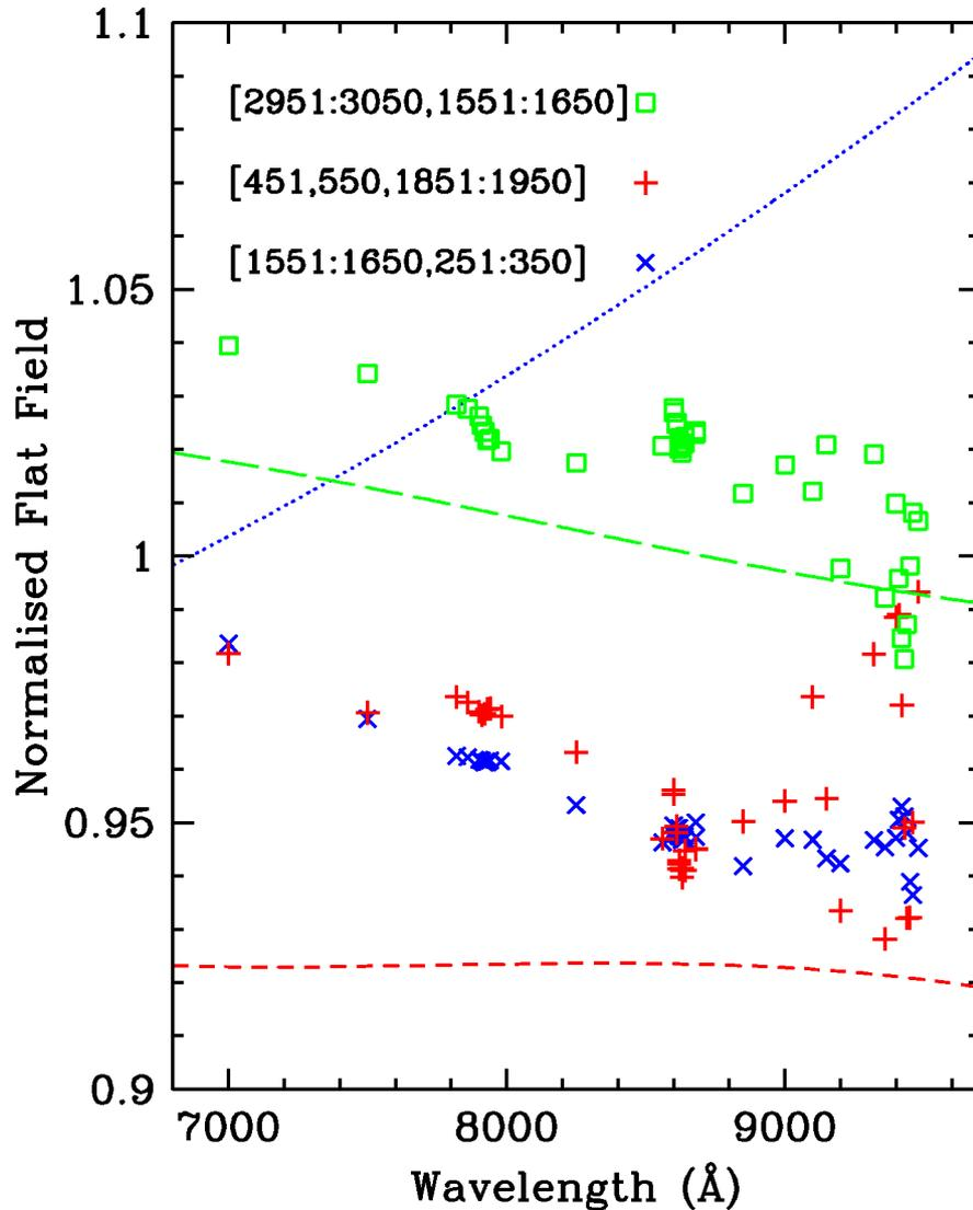
**Figure 5:** For WFC CHIP1 the points from the normalised ground flat-fields in the apertures listed are compared with the fits (lines) from the in-orbit flat-fields for the same areas. The points and lines are colour-coded to distinguish the values for the same aperture.
