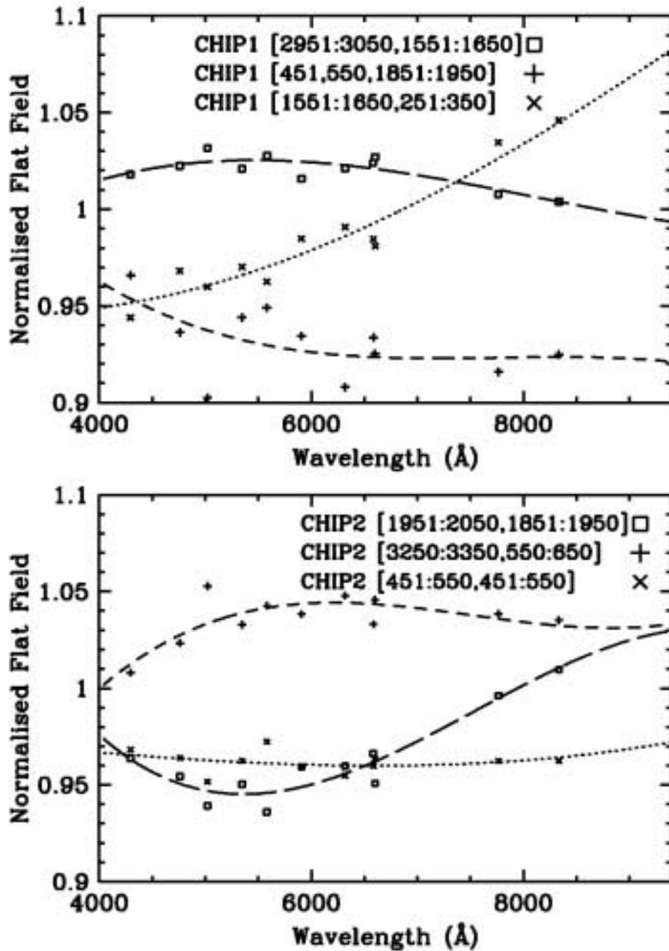
**Figure 3:** The mean values in square apertures for the in-orbit flat-fields with the WFC, are plotted as a function of wavelength. The flat-field values correspond to regions which are listed in the figure and 3rd order polynomial fits are shown by lines.
