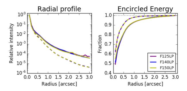
**Figure 3:** Comparison between observed (solid lines) and Tiny Tim (dashed lines) radial profiles and encircled energy curves. Tiny Tim models of the three filters are so close to each other that they overlap in this figure.
